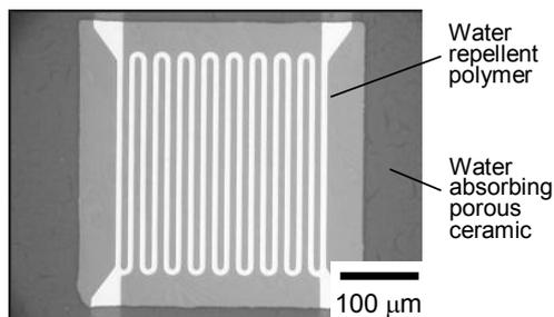
Fig. 3: Microheater covered with water-repellent polymer and surrounded by water-absorbing porous ceramics.
