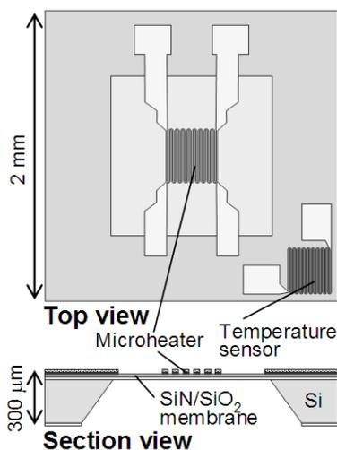
Fig. 1: Structure of heat transfer type H<sub>2</sub> sensor.
