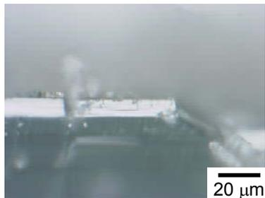
Fig. 8: No visible residual water droplet in the microgap on water-droplet-removal structure 2 just after injection of water droplets.
