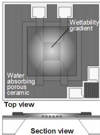
Fig. 6: Water-droplet-removal structure 3: Wettability gradient between the inner (hydrophobic) and outer (hydrophilic) area eliminates water droplets from the sensing area.
