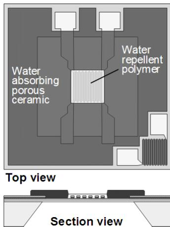
Fig. 2: Water-droplet-removal structure 1: The center and surrounding areas of the H<sub>2</sub> sensor are coated with water-repellent polymer and water-absorbing porous ceramics, respectively.
