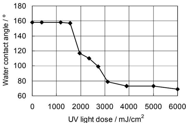
Fig. 10: UV light dose dependency of water contact angle on the photochromic compound coating.
