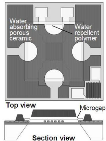
Fig. 4: Water-droplet-removal structure 2: The porous ceramics is placed above the water-repellent polymer on the inner area of the H<sub>2</sub> sensor, with a microgap in between.
