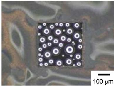
Fig. 7: Remaining water droplets on water-droplet-removal structure 1.
