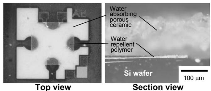
Fig. 5: Water-absorbing porous ceramics structure on water-repellent polymer coating with a microgap.
