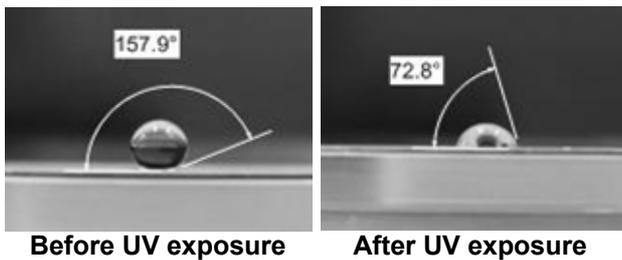
Fig. 9: Water droplets on photochromic compound deposited on super-water-repellent undercoat before and after UV exposure.
