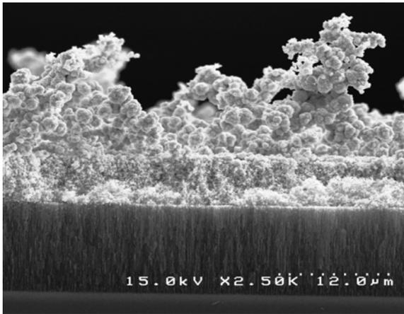
Fig.2: The cross-sectional view of porous Pd layer using PdCl<sub>2</sub> plating bath
