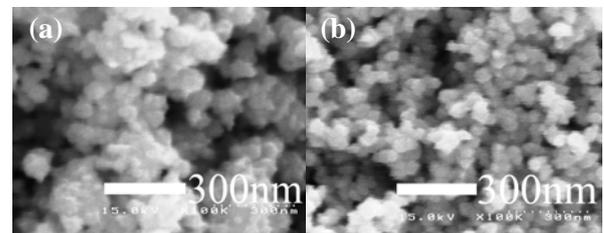
Fig.4: Comparing the particle of Pd. (a) Using PdCl<sub>2</sub> bath, (b) Using ethylenediamine complexation bath
