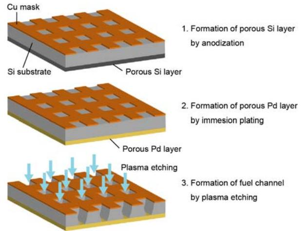
Fig.6: Fabrication process of the monolith electrode.
