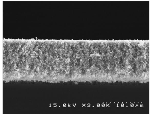
Fig.3: The cross-sectional view of porous Pd layer using ethylenediamine complexation bath
