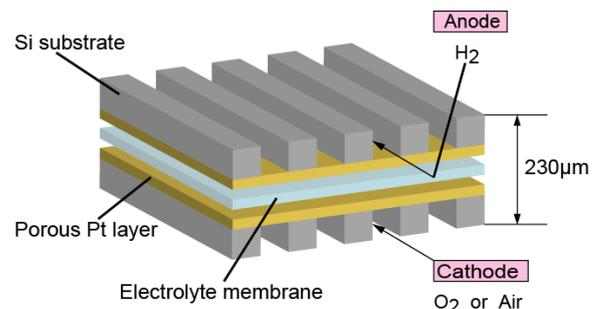
Fig.1: Schematic view of the Si based fuel cell
