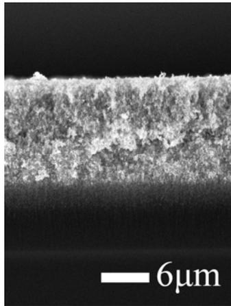
Fig.5: The cross-sectional view of porous Pd layer
