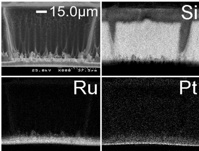
Fig. 4: Cross sectional view obtained by SEM and EDS elemental mapping of the through-chip Ru-Pt catalyst layer.
