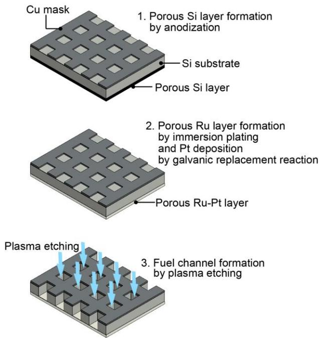
Fig. 2: Fabrication process of the monolithic electrode.
