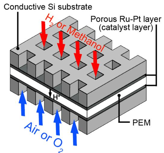
Fig. 1: Schematic view of the Si based fuel cell.
