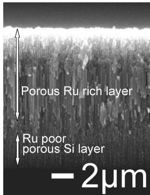
Fig. 6: Cross sectional view of the porous Ru-Pt catalyst layer.
