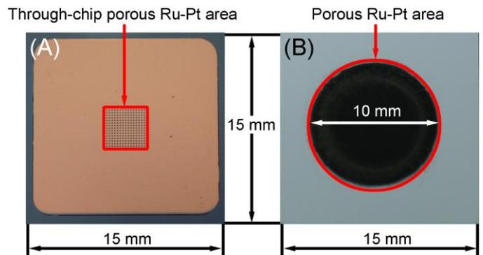
Fig. 3: Photograph of specimen chip – (A)Cu mask surface, (B)Porous Ru-Pt layer surface.
