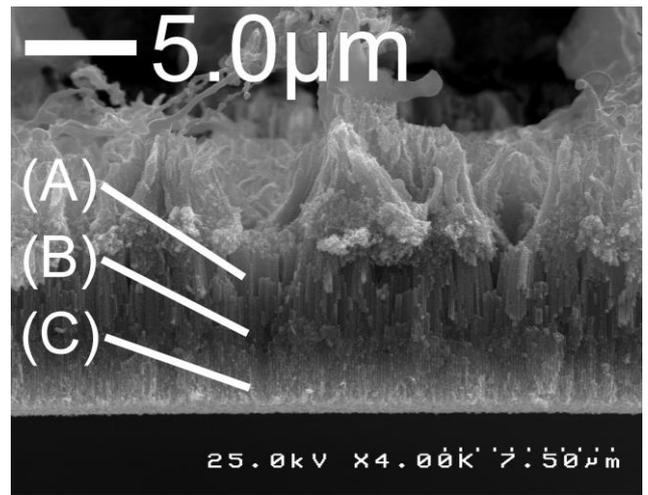
Fig. 5: Magnified view of the porous Ru-Pt catalyst layer.
