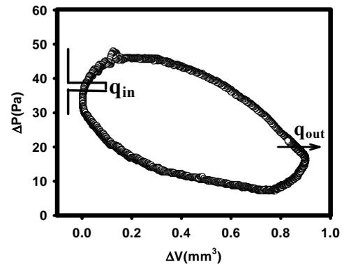
Fig.3: Measured P-V diagram for resonant engine.
