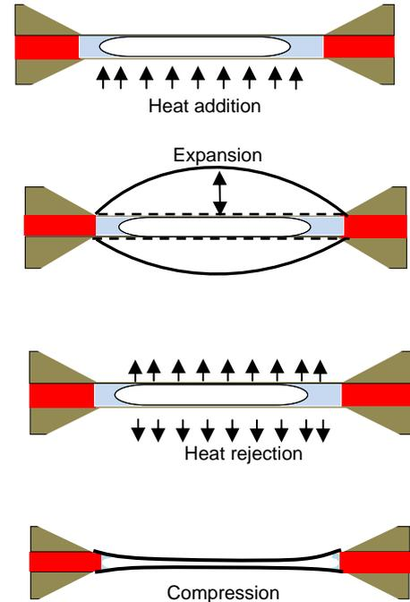
Fig. 2: Working cycle of micro heat engine.
