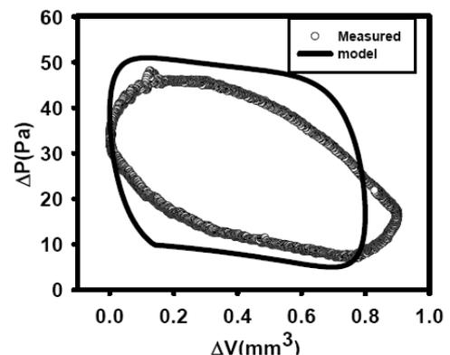
Fig. 5: Comparison of modeled and measured P-V diagram.
