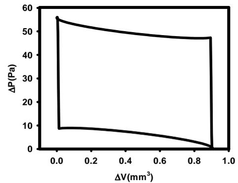
Fig. 4: Modeled P-V diagram for resonant engine.
