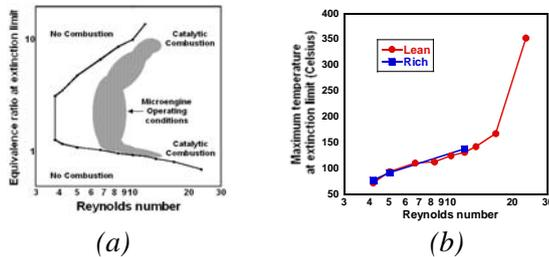
Fig. 2: (a) Extinction limit map for catalytic combustion, (b) Maximum combustor temperatures ( $T_{max}$ ) at lean and rich extinction limits.
