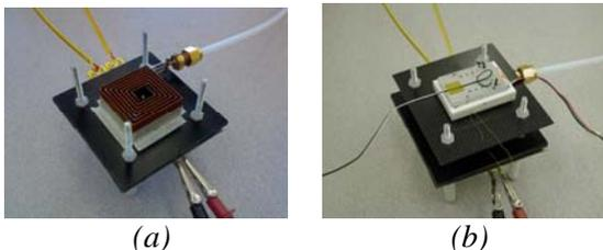
Fig. 1: (a) CNC-milled Swiss roll combustor; top plate removed for clarity, and (b) micro-engine mated with Swiss roll combustor in experimental stand.
