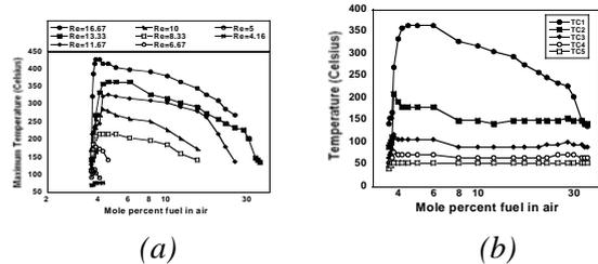
Fig. 3: (a) Maximum combustor temperatures ( $T_{max}$ ) as a function of Re and mixture strength, (b) temperature profiles recorded over a range of mixture compositions at Re = 13.33.
