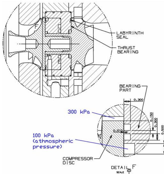
Fig. 3 Section view of air bearing unit and labyrinth seal detail view.
