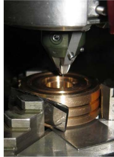
Fig. 4 Production of the feedholes by  $\mu\text{EDM}$  technology.
