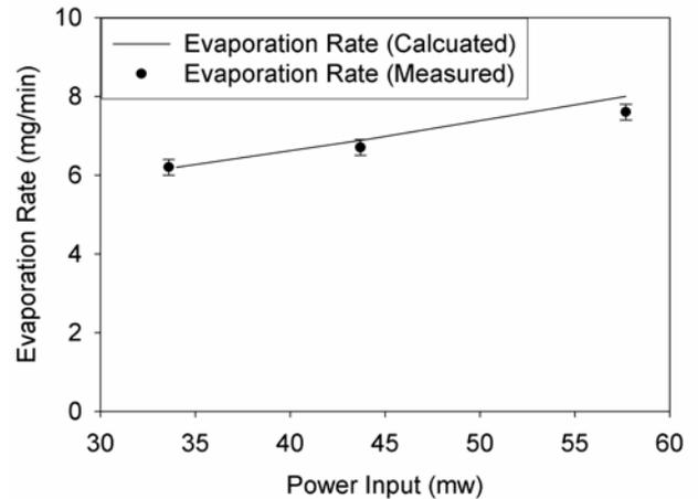
Figure 5. Evaporation rate from the Si microchannel evaporator versus power input.
