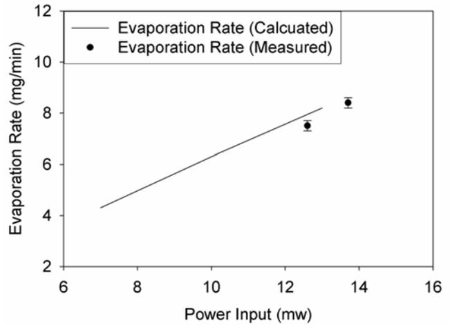
Figure 7. Evaporation rate from the SiNx microchannel evaporator versus power input.
