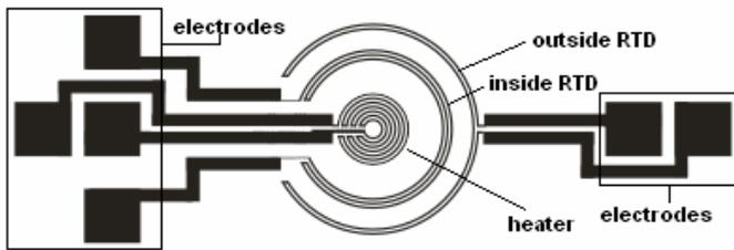
Figure 2. Experimental test die schematic.
