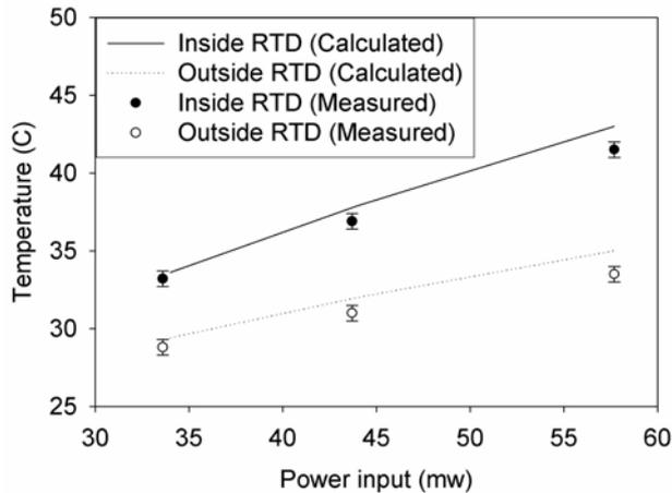
Figure 4. Temperature distribution in the Si microchannel evaporator versus power input.
