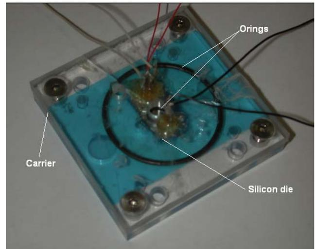
Figure 3. Photograph of microchannel evaporator die in its acrylic carrier.
