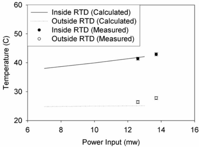
Figure 6. Temperature distribution in the SiNx microchannel evaporator versus power input.
