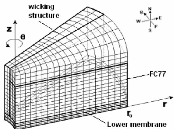
Figure 1. Schematic of axisymmetric numerical model
