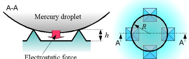
Figure 5. Diagram for estimating the maximum driving voltage.
