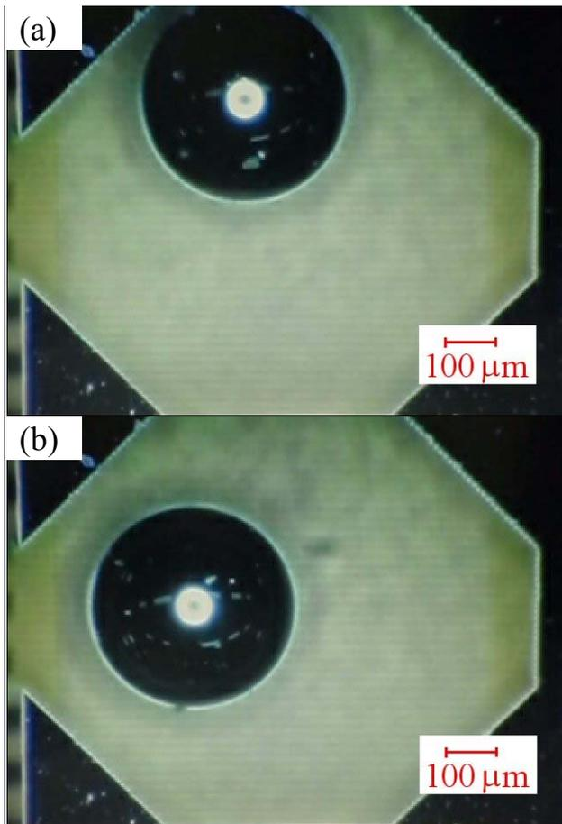
Figure 8. Actuation result: (a) Initial state, (b) Final state, in which the droplet was trapped.
