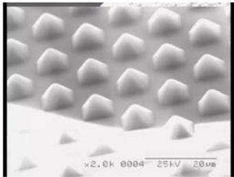
Figure 1. SEM image of micro pillars.
