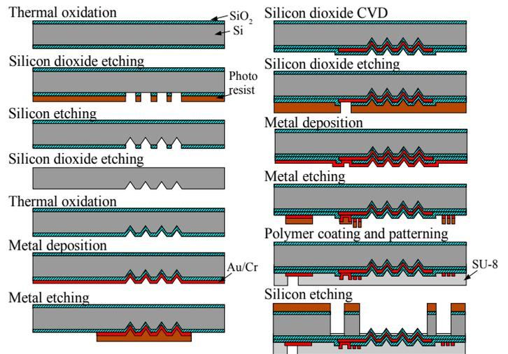
Figure 6. Fabrication process.
