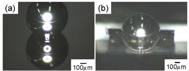
Figure 2. Mercury droplet on (a) a flat silicon dioxide and (b) micro pillars.
