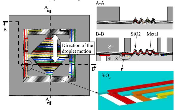
Figure 3. Structure of the mercury droplet actuator.
