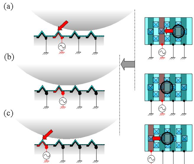
Figure 4. Droplet working mechanism: (a) An energized electrode attracts the droplet. (b) The droplet moves by a pitch of driving electrodes. (c) The next electrode is energized and attracts the droplet again.
