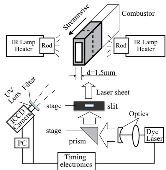
Fig. 8: Schematic of experimental setup for OH-PLIF.
