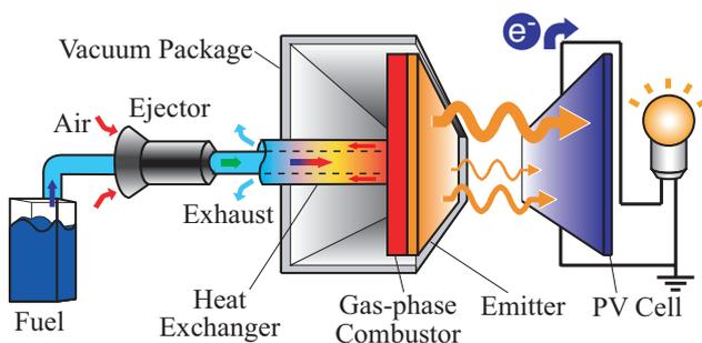
Fig. 1: Schematic of micro TPV system concept.
