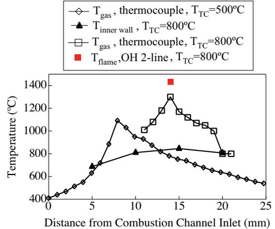
Fig. 10: Gas/flame temperature at the combustion channel centre-line.
