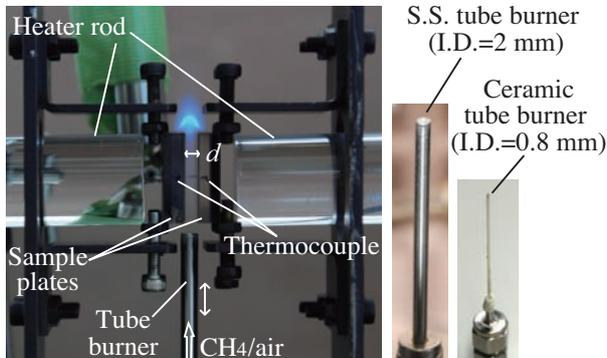
Fig. 3 Magnified view of the experimental setup for quenching distance measurement and tube burners.
