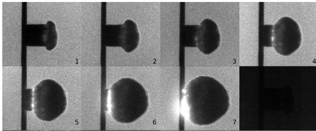
Fig. 5: Direct laser irradiation results in shorter ignition delay. 50ns inter-frame, 10 ns exposure.
