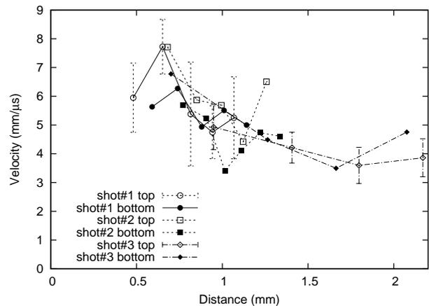
Fig. 7: Velocity profiles measured at top and bottom surface of a cylindrical pellet.
