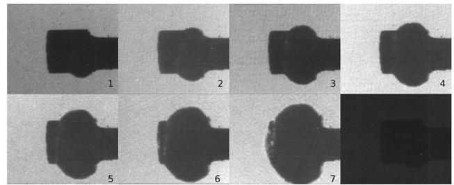
Fig. 6: Shadowgraph images of detonation propagation in a  $AgN_3$  pellet. 25 ns inter-frame, 5 ns exposure.
