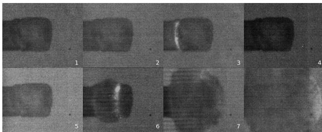
Fig. 2: From laser irradiation to explosion of a  $AgN_3$  pellet. 200 ns inter-frame, 50 ns exposure per frame.
