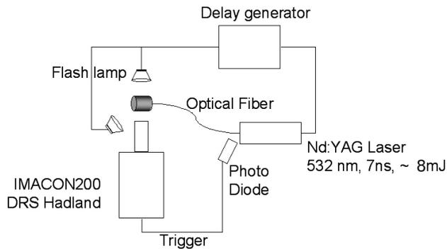
Fig. 1: Schematics of experimental setup
