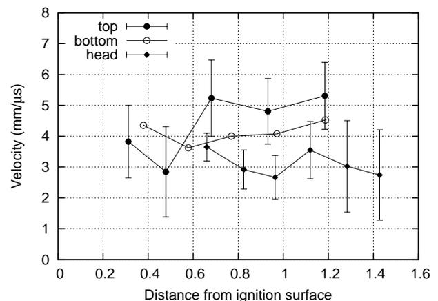
Fig. 8: Velocity profiles of detonation front by direct laser irradiation.
