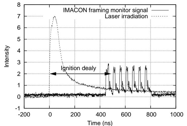
Fig. 4: Framing monitor signal of IMACON200 and photodiode output detecting laser irradiation.
