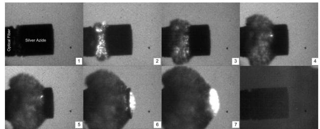
Fig. 3: Detonation propagating in a  $AgN_3$  pellet of 1.5 mm diameter. 50ns interframe, 25ns exposure.
