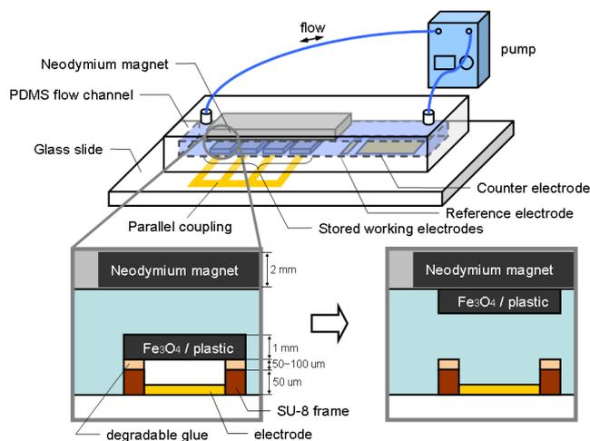
Fig. 2: Prototype of miniature biofuel cells.
