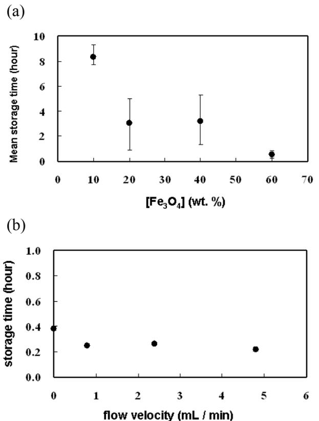
Fig. 5: Parameters affecting to storage time of electrodes (a) the mixture ratio of  $\text{Fe}_3\text{O}_4$ , (b) the flow rate. The measurements were performed three times in the phosphate buffer (pH 7) containing 5 mM  $\text{K}_3[\text{Fe}(\text{CN})_6]$ , 0.1 M NaCl, at room temperature, with a flow rate of  $0.8 \text{ mL min}^{-1}$  (a).
