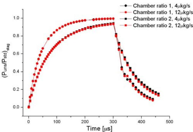
Fig. 6: Change of normalized stagnation pressure with time for different mass fluxes (colors) and chamber volumes (symbols).
