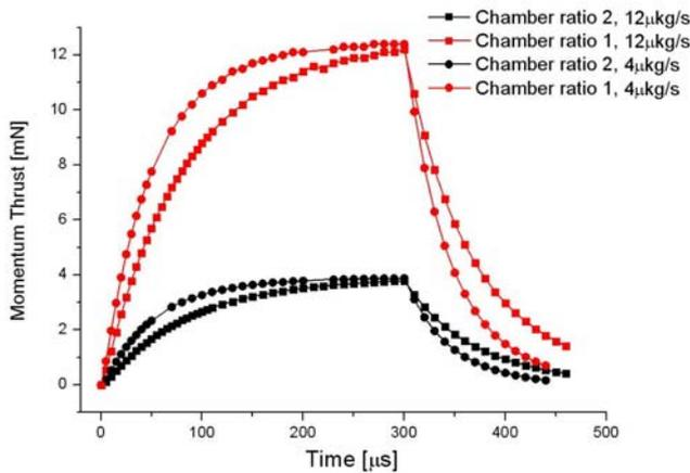
Fig. 5: Change of momentum thrust with time for two different chamber volumes at two different mass fluxes.
