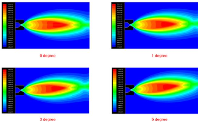
Fig. 8: Mach contours for the distorted nozzle.
