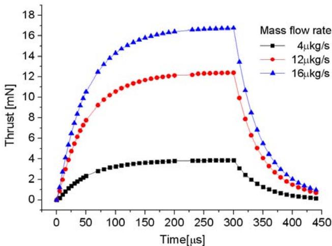
Fig. 2: Change of thrust with time for three different mass input fluxes.
