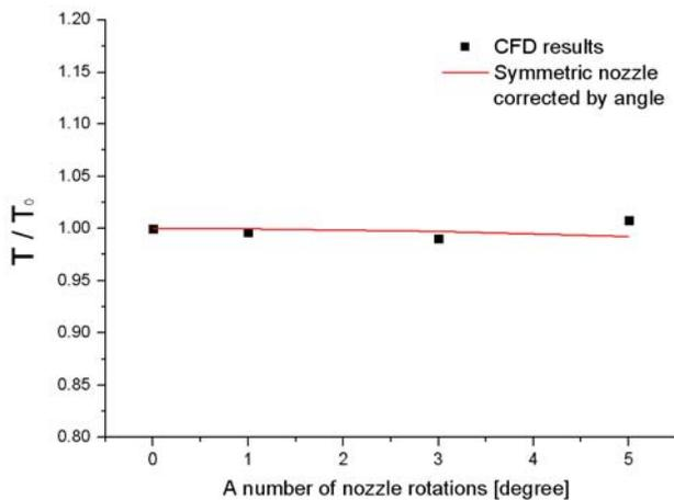
Fig. 9: Thrust in the x-direction for a number of nozzle axis rotations (symbols), normalized to that of the symmetric case and corrected for the angle (line).
