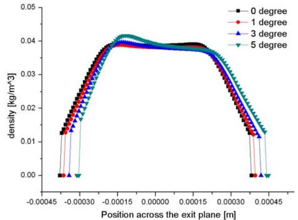
Fig. 10: Profile of x-velocity and density at the exit plane for a number of nozzle axis distortions.
