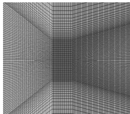
Fig. 1: Schematic of the grids near the nozzle throat.
