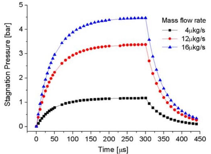
Fig. 3: Change of chamber pressure with time for three different mass input fluxes.
