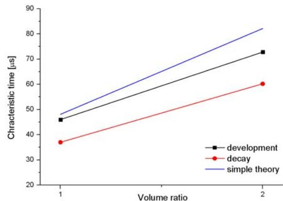
Fig. 7: Comparison of the calculated characteristic time (symbols) and simple theoretical model (line) for two different chamber sizes.
