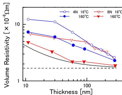
Fig.4 the volume resistivity on the films with different thickness.
