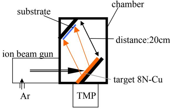
Fig.1 scheme of the copper thin film processing.
