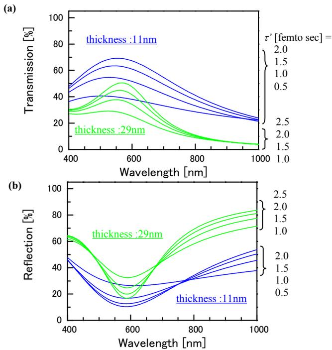
Fig.5 Calculated transmission and reflection spectrum on copper films.
