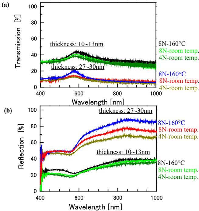
Fig.6 Measured transmission and reflection spectrum on the copper films.
