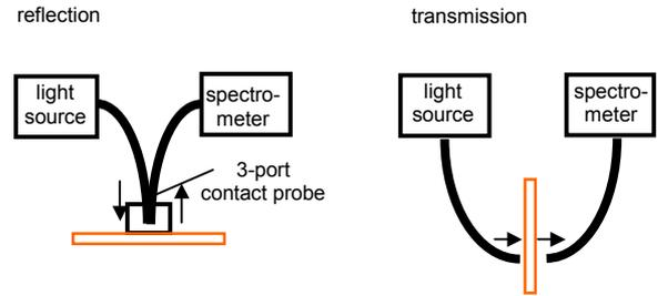
Fig.2 Measurement setup of optical properties.
