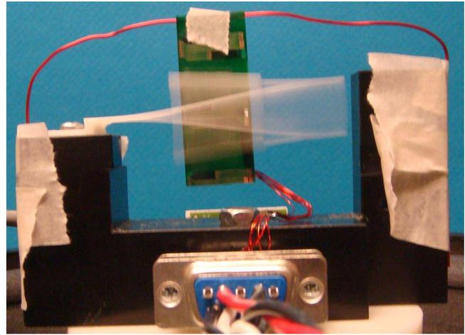
Figure 3: resonating generator on a shaker table.
