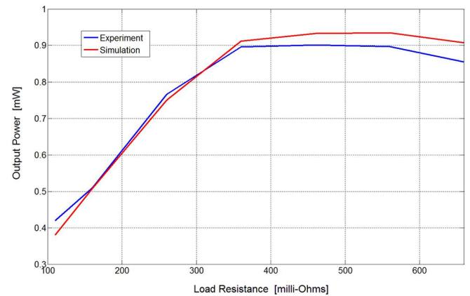
Figure 6: total generator output power.
