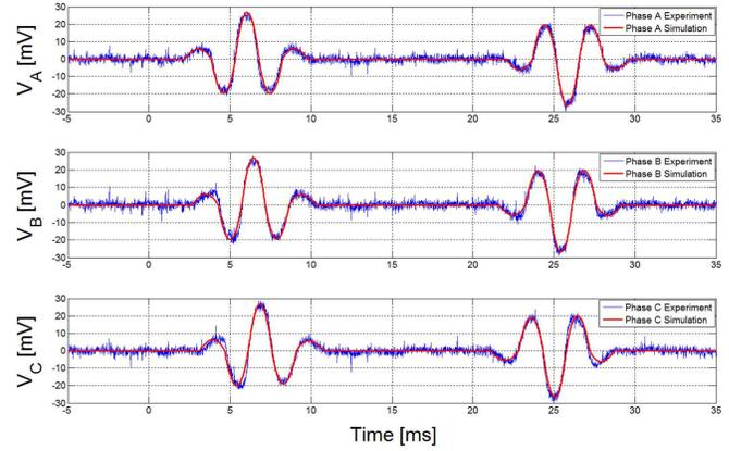
Figure 5: loaded generator voltage waveforms.
