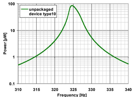
Fig. 1. An unpackaged device type 10 generates 85  $\mu\text{W}$  at an excitation of 1.75 g at atmospheric pressure.
