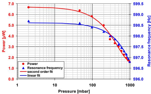
Fig. 6. Power and resonance frequency versus pressure for an unpackaged device of type 5 at an acceleration of 0.2 g.
