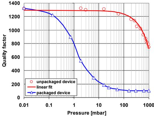
Fig. 4. The measured quality factors as a function of pressure. The unpacked device is hindered by viscous damping; the package device by squeeze film damping.
