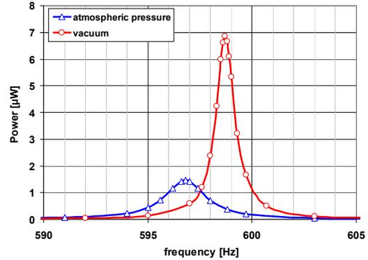
Fig. 5. Resonance curves of an unpacked device of type 5 at 0.2 g at atmospheric pressure and at vacuum showing an increase in power.
