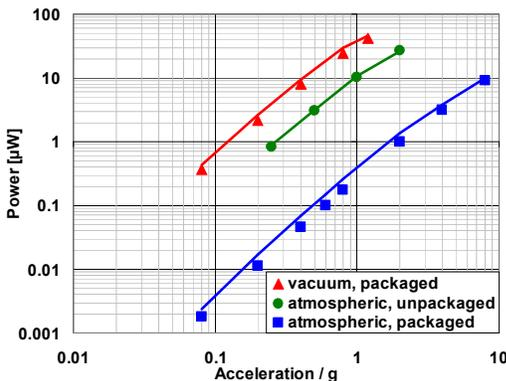
Fig. 7. Measured (dots) and modeled (lines) power as function of acceleration for a device type 3. The highest power is generated with a vacuum package.
