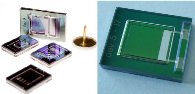
Fig. 3. Photograph of vacuum packaged vibration energy harvesters (left) and a close up (right) of a device showing the glass cap and contact openings.
