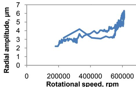
Fig. 9: Radial amplitude of rotor vibration as a function of rotation speed
