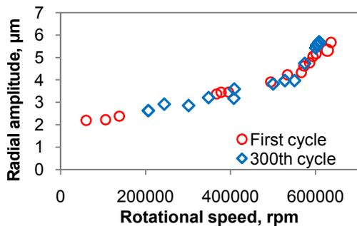
Fig. 11: Radial amplitude of rotor vibration in the first and three hundredth start-and-stop cycle
