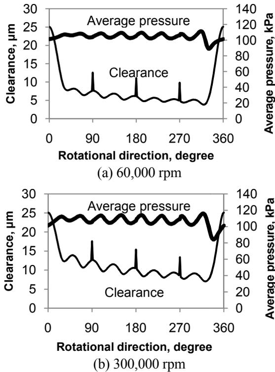
Fig. 6: Calculated bearing clearance and pressure averaged along the axial direction
