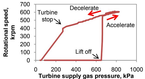
Fig. 8: Relationship between turbine supply pressure and rotation speed
