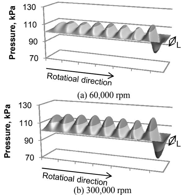
Fig. 5: Simulated pressure distribution in the bearing clearance
