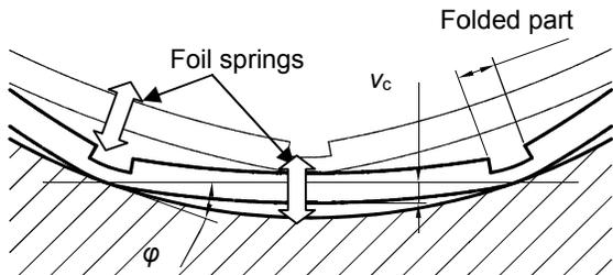
Fig. 2: Schematic of the foil in the housing
