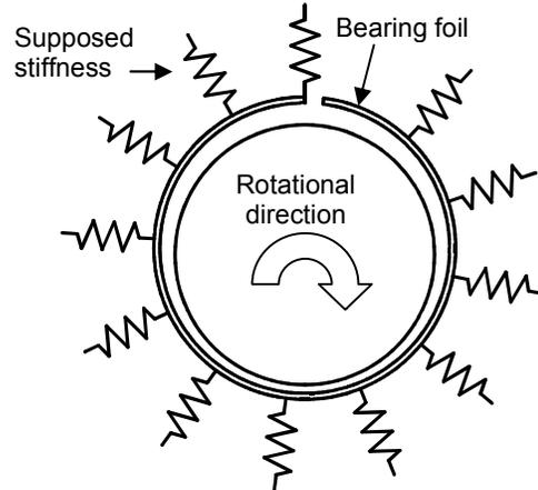
Fig. 4: Calculation model of the foil bearing
