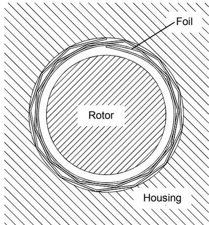
Fig. 1: Structure of a tape type foil bearing
