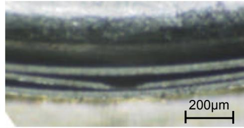
Fig. 3: Micrograph of the foil in the housing
