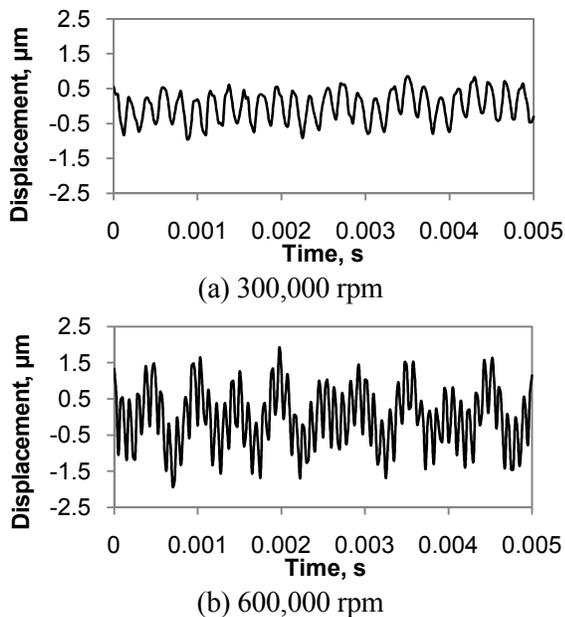
Fig. 10: Waveform of radial rotor vibration
