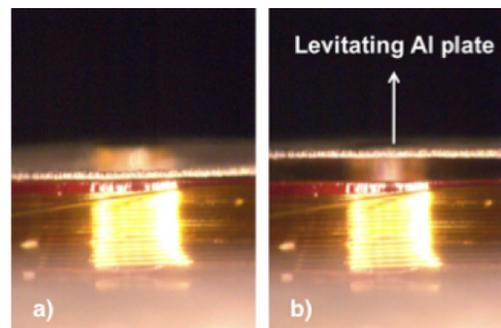
Figure 3: Side view optical micrograph of the levitation micro-coil and the Al plate: a) no signal is applied to the levitation micro-coil: the Al plate is in contact with the SU8 post supporting the micro-coil; b) AC signal is applied to the levitation micro-coil: the Al plate is levitated to a height of approx. 90 $\mu\text{m}$ .
