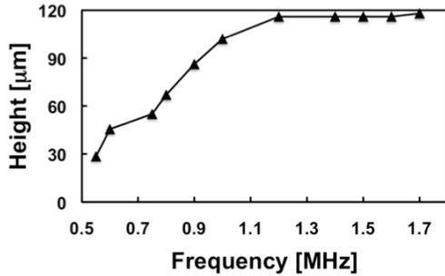
Figure 4: Levitation height versus excitation frequency of a  $2700\mu\text{m}$  diameter Al plate on top of a  $2500\mu\text{m}$  diameter coil. The amplitude of the signal was  $20V_{pp}$ .
