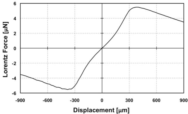
Figure 5: Simulation of the lateral Lorentz force component in the first generation magnetic micro-bearing structure
