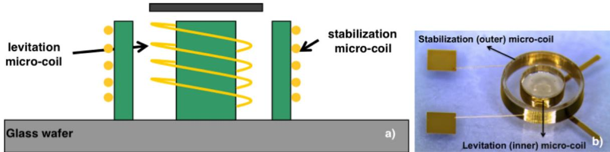
Figure 2: Magnetic micro-bearing with secondary stabilization micro-coil, a) schematic, b) photo.
