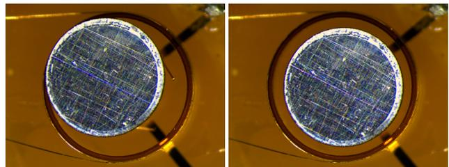
Figure 7: a) Top view of the Al plate off-center before applying signal to the stabilization micro-coil; b) Top view of the successfully centered Al plate upon applying  $2.2\text{MHz}$ ,  $20V_{pp}$  signal to the stabilization micro-coil.
