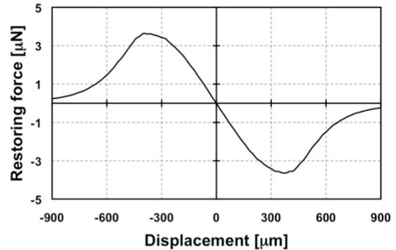
Figure 6: Restoring force as a function of the off-center displacement for a  $1500\mu\text{m}$  diameter levitation micro-coil and  $700\mu\text{m}$  gap between the levitation and stabilization micro-coils. The displacement and the force have opposite signs, thus the force acts as a restoring force.
