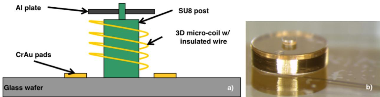
Figure 1: Magnetic micro-bearing structure with center pin stabilization: a) schematic, b) photo.
