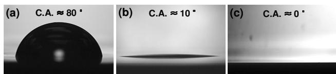
Fig. 2: Optical images of droplets (4 $\mu\text{l}$ ) of the electroplating solution on the photoresist layers. (a) before plasma treatment, after 2 min plasma treatment (b) and 10 min treatment (c).
