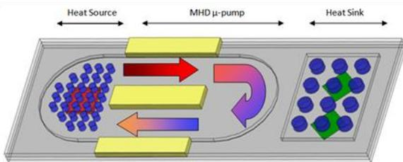
Figure 1: CAD depicting the configuration of a micro-cooling system using the MHD  $\mu$ -pump
