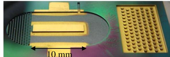
Figure 2: MHD  $\mu$ -pump fabricated using Silicon MEMS technology with Gold electrodes and micro-pin heat-exchangers
