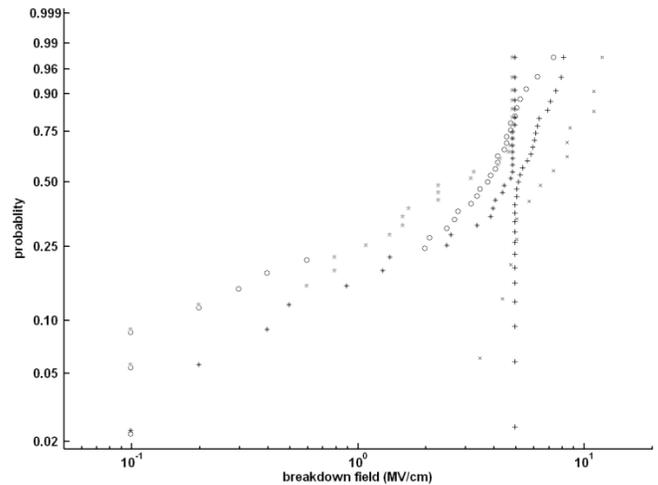
Figure 5. Weibull of probability breakdown field for MIM built on planar Si/SiO<sub>2</sub> (+), first anodized Al (O), 500nm (□) and 2 $\mu\text{m}$  (◇) structures.
