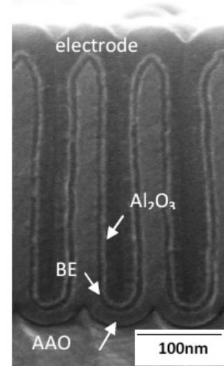
Figure 3. SEM cross section of 500nm MIM capacitors in AAO templates.
