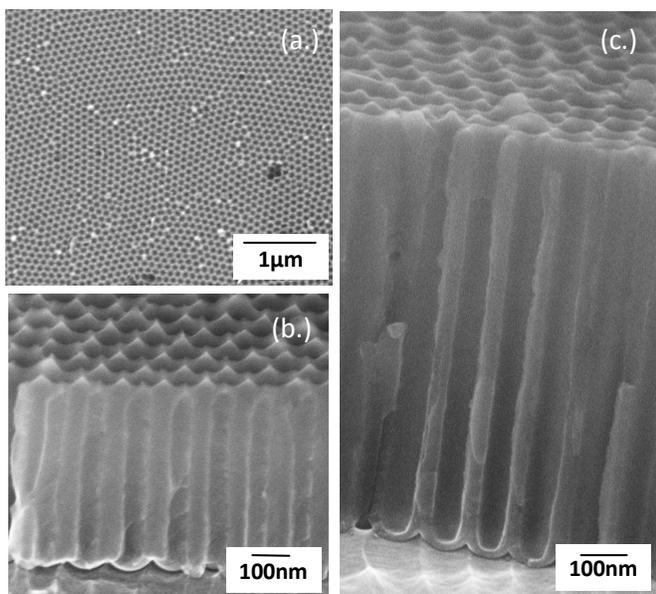
Figure 6. a) first anodized Al surface b) 500nm pores without RIE etch shows sharp peaks and c) 1μm pore with RIE etch shows rounded peaks.
