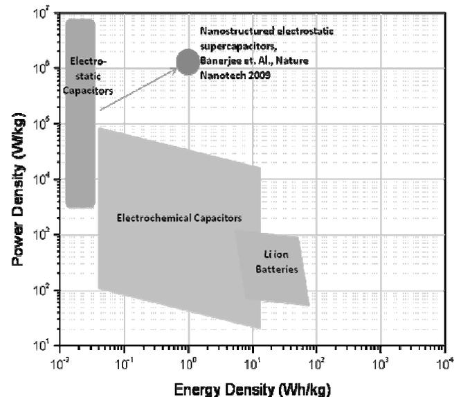
Figure 1: Ragone Plot shows MIM high energy density and high power density.
