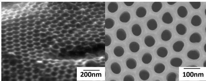
Figure 2. SEM images of first anodized Al surface (left) and top-view of pore-widened AAO (right).
