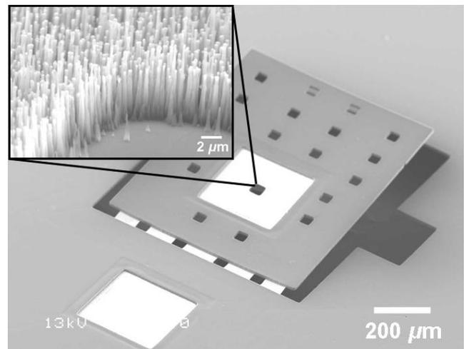
Fig. 3: SEM image of a CNT-origami supercapacitor prior to folding. The inset shows the CNT-covered electrode surface.
