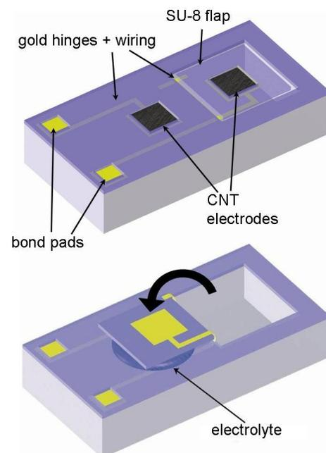
Fig. 1: Schematic of the CNT-origami supercapacitor before and after the folding process.
