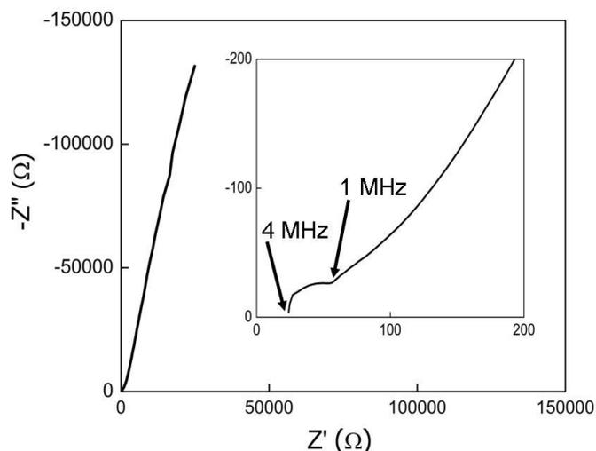
Fig. 5: Nyquist plot of the EIS results shown for frequencies between  $4 \text{ MHz}$  and  $4 \text{ Hz}$ .
