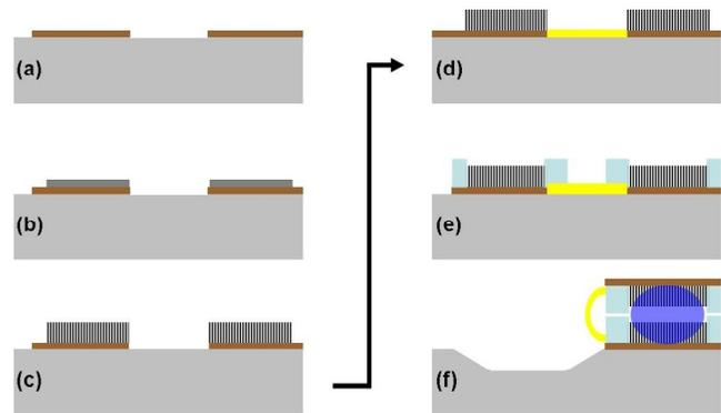
Fig. 2: Process flow for the CNT-origami electrochemical capacitor. (a) Deposit/pattern TiN layer. (b) Deposit/pattern catalyst layer. (c) Grow CNTs. (d) Deposit/pattern Au layer through lift-off. (e) Deposit/pattern SU-8 layer. (f) Release membrane, deposit electrolyte, and fold over flap.
