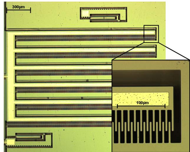
Fig. 3: Photograph of the fabricated micro capacitive energy harvester.
