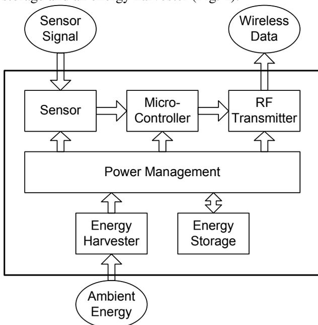
Fig. 1: Components of an autonomous system which is powered by energy harvesting.
