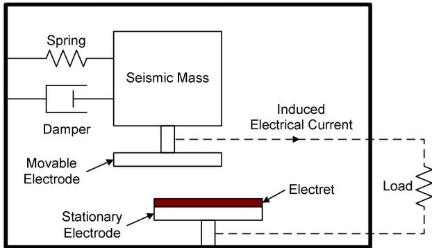
Fig. 2: Schematic view of capacitive harvester model.
