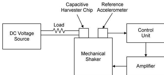
Fig. 5: Schematic of the measurement setup
