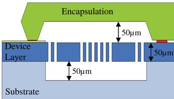
Fig. 4: Cross section view of the capacitive energy harvester chip.
