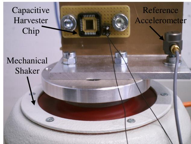
Fig. 6: Photograph of capacitive harvester chip and reference accelerometer mounted on the mechanical shaker.
