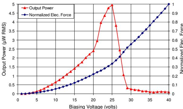
Fig. 9: Electrical output power and the normalized electrostatic force.
