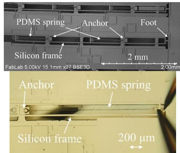
Figure 1: Micromechanical thruster
