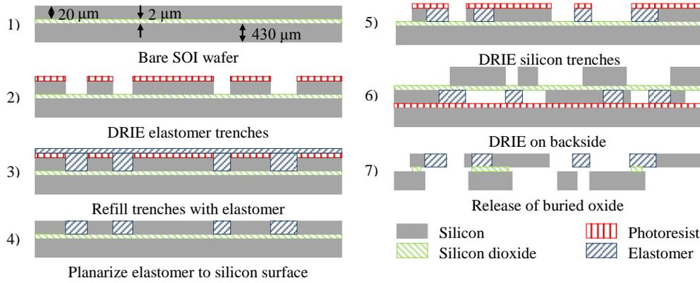
Figure 2: Microfabrication Process
