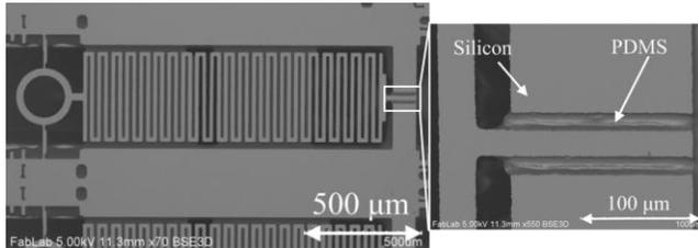
Figure 4: SEM of test structure used to test shear adhesion
