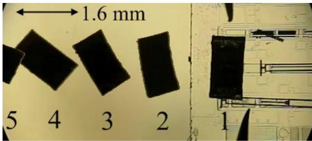
Figure 7: A thruster propelling a 2 mg resistor
