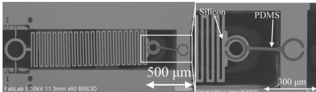
Figure 5: SEM of test structure used for stress-strain
