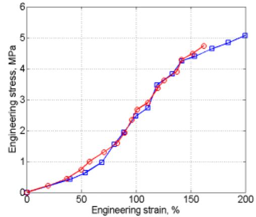
Figure 6: Measured stress-strain for PDMS
