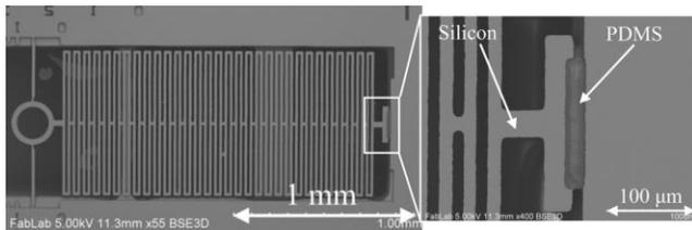
Figure 3: SEM of test structure used to test normal adhesion
