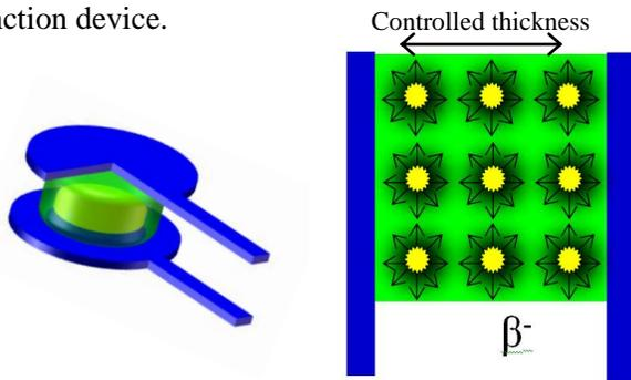
Fig. 4: The encapsulated design for betavoltaic.
