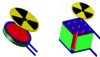
Fig. 1: 3D view of the conventional betavoltaics (a) planar structure (b) porous structure.
