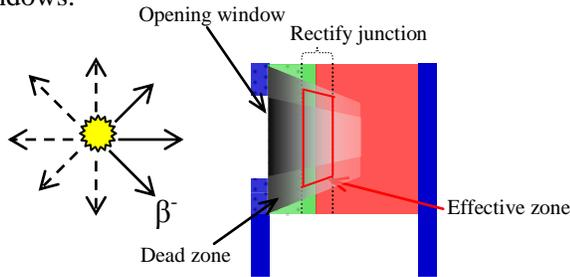
Fig. 2: The schematics illustrating the losses mechanism of emitted beta particles
