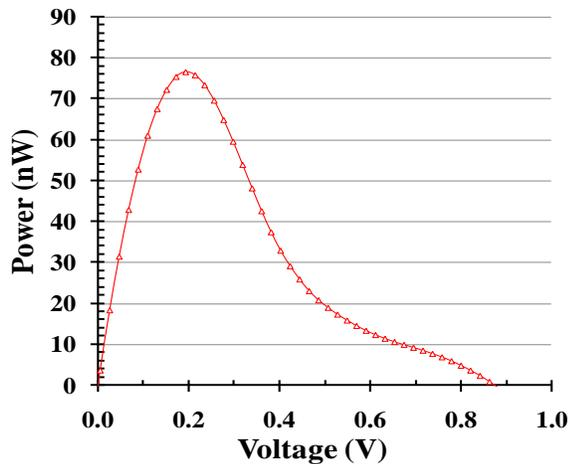
Fig. 6: Output power against the bias voltage
