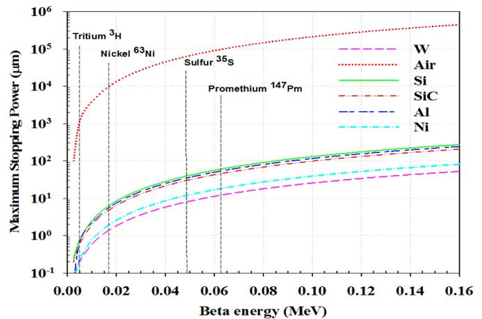
Fig. 3: Maximum stopping power of beta particles in different materials with the average beta energy from variety of radioactive ( $^3\text{H}$ ,  $^{63}\text{Ni}$ ,  $^{35}\text{S}$ , and  $^{147}\text{Pm}$ ).
