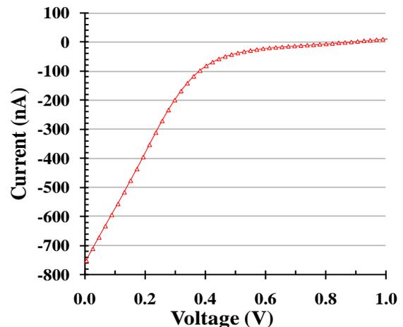
Fig. 5: The I-V characteristic of encapsulated device at room temperature
