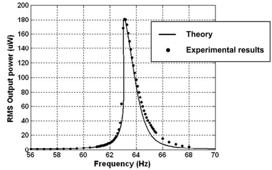
Fig. 7: Output power of the piezoelectric generator.
