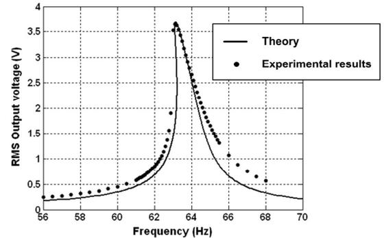
Fig. 8: Output voltage of the piezoelectric generator.
