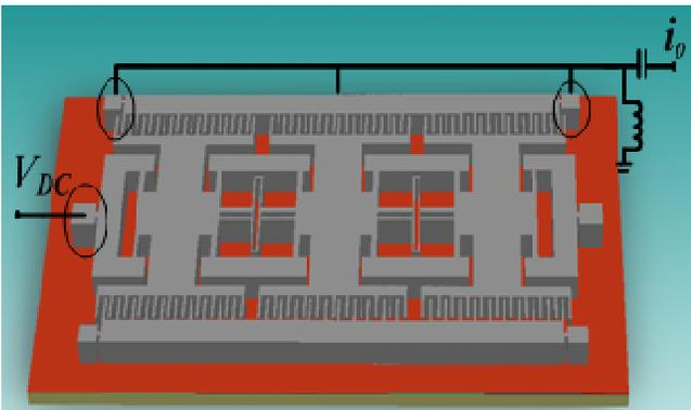
Fig. 1: 3-dof harvester with amplified bandwidth.
