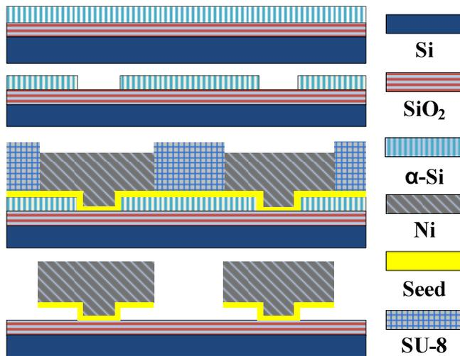
Fig. 5: The fabrication process of energy harvesters.
