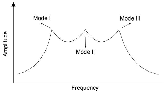
Fig. 4: The frequency response function of the coupled harvesters.
