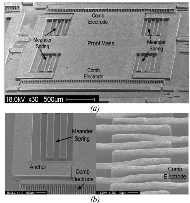
Fig. 6: (a) and (b) SEM pictures of fabricated energy harvesters.
