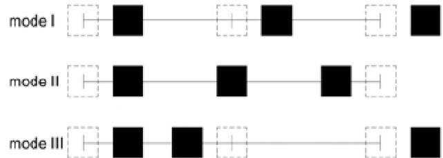
Fig. 3: Modal displacements of 3-dof harvesters.
