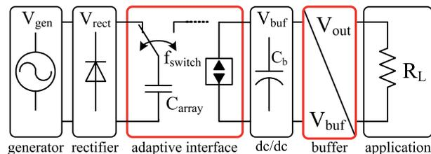
Fig. 1: An adaptive interface is required between rectification and storage.
