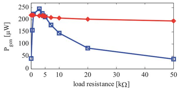
Fig. 11: Generator output power with (diamonds) and without (squares) the adaptive interface chip.
