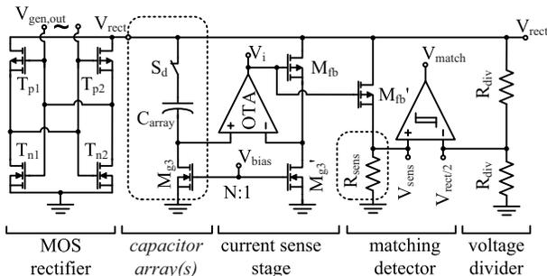
Fig. 7: Schematic shows load matching detector between the rectifier and array capacitors.
