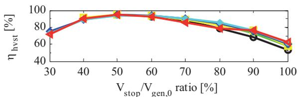
Fig. 9: The charging power and harvesting efficiency passes a maximum as charge stop level is increased.
