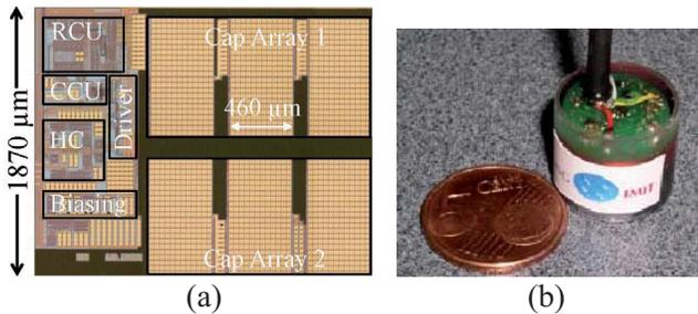
Fig. 3: Micro photography of the interface chip (a) and the inductive generator (b).
