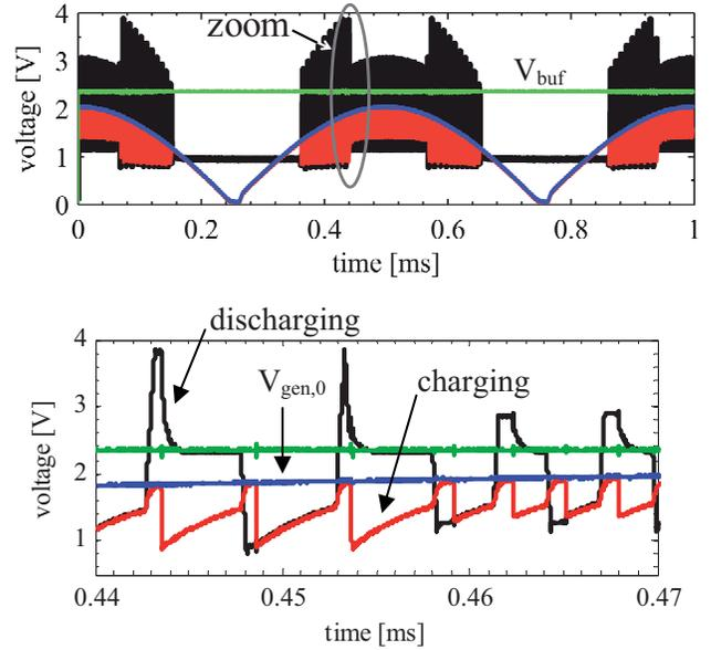
Fig. 5: Measured transient waveforms (a) of the impedance matching interface, also with zoom (b).
