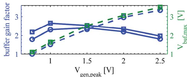
Fig. 10: Maximum buffer voltage due to stacking and resulting increase of buffered energy.
