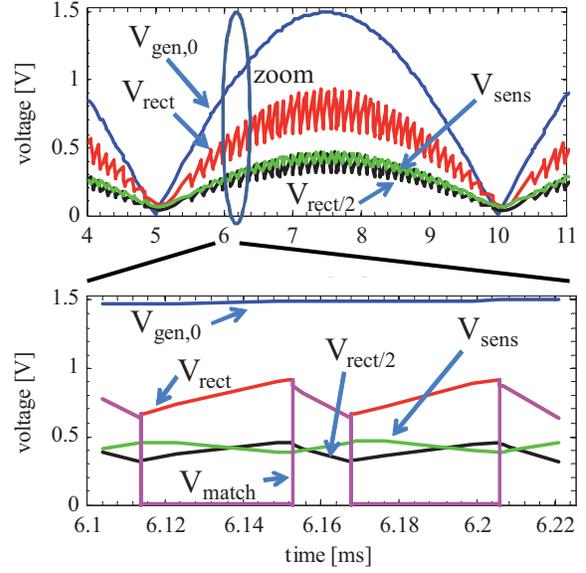
Fig. 8: (a) Simulations of the generator output voltage  $V_{\text{gen}} (\approx V_{\text{rect}})$ , which ripples around  $1/2 V_{\text{gen},0}$ , and (b) the zoomed view of the load matching detection – with delayed comparator signal  $V_{\text{hc}}$ .
