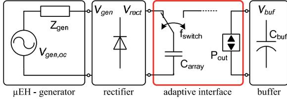
Fig. 2: Load matching interface presents a charge controlled and toggling capacitance to the generator.
