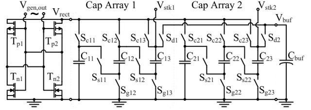
Fig. 4: Switched capacitors of the interface are located between the rectifier and the buffer.
