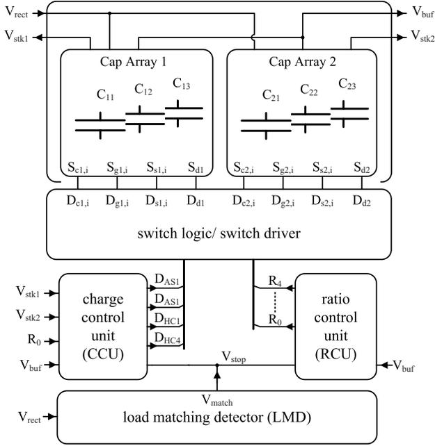
Fig. 6: Building blocks of the adaptive interface chip with added load matching detector.
