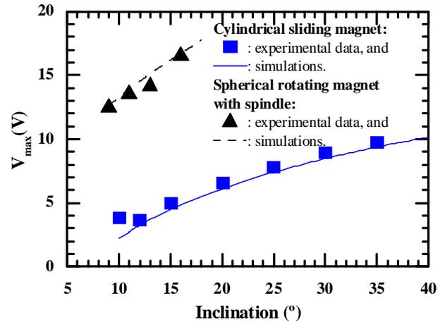
Fig. 4: maximum open circuit output voltage, generated through a single coil as a function of the inclination angle for both types of device.
