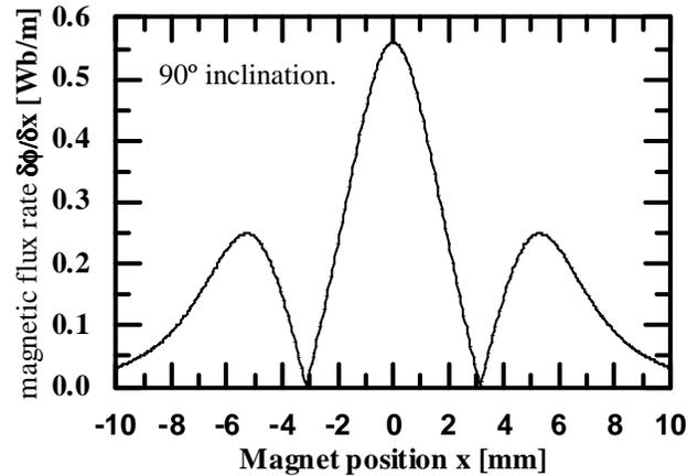
Fig. 2: Flux rate distribution created by a sliding spherical magnet along a tube with two optimized coils (assuming optimum magnet orientation along whole displacement).
