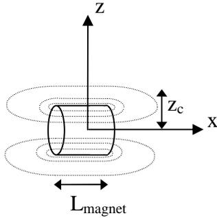
Fig. 6: Schematics of the filling critical distance  $z_c$ .
