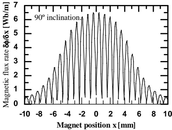
Fig. 3: Flux rate distribution along a tube with two optimized coils from a rotating spherical magnet with a magnet/spindle size ratio of 10.
