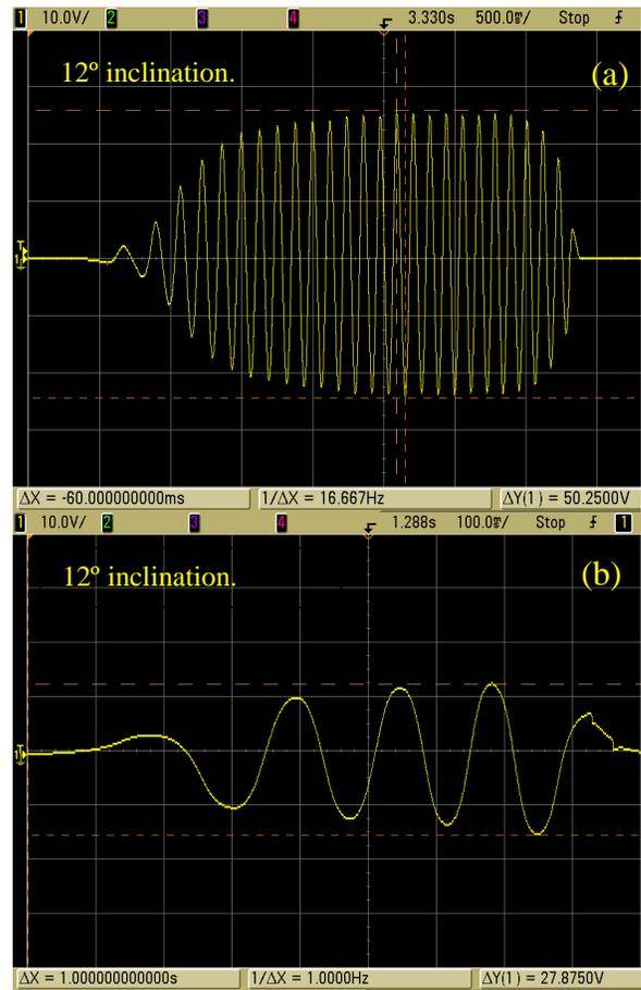
Fig. 5: Open circuit output voltage for a) spindle design, and b) sliding magnet design.
