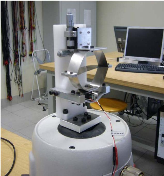
Fig. 8: Experimental NLBO mounted on a test rig.
