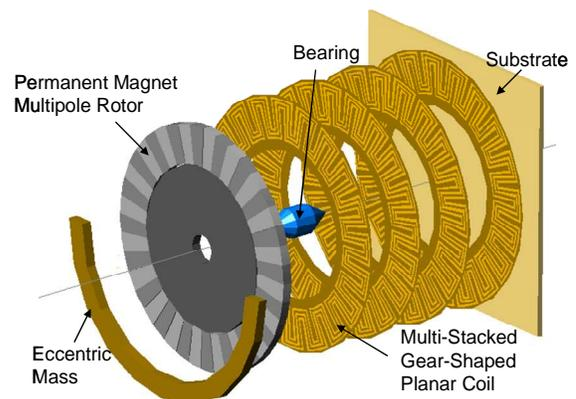
Fig. 1: Simplified schematic of the proposed design.
