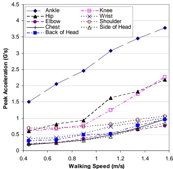
Fig. 2: Peak acceleration on several body locations while walking at different speeds on a treadmill ( $1G=9.8\text{m}/\text{s}^2$ ).
