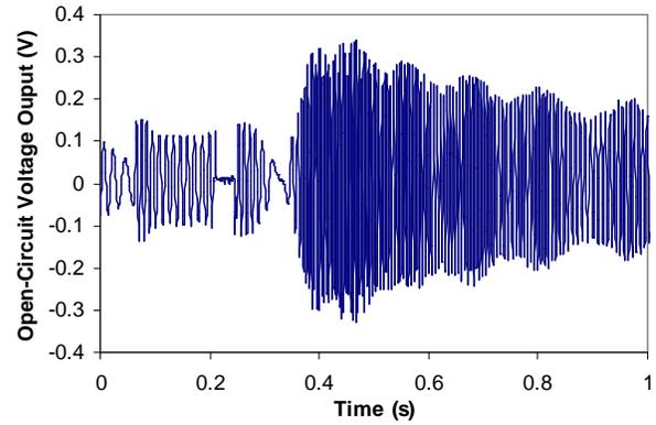
Fig. 6: Open-circuit voltage while walking with the generator laterally placed on the ankle for the 2-layer coil test (200 µm line width and 4 turns) and 20 discrete NdFeB PM pole-pairs (1.1x1.1x5.1mm). A peak voltage of 326mV was reported (70mV<sub>rms</sub>).
