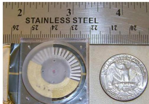
Fig. 3: Two-rotor meso-scale prototype. Rotor with 20 pole-pairs of NdFeB PM ( $1.1 \times 1.1 \times 5.1\text{mm}$ ) and a jewel bearing design (bottom rotor not shown).
