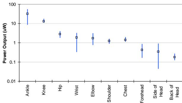
Fig. 5: Average, minimum and maximum power output for a 2-layer coil generator placed on different body locations while walking (seven tests).
