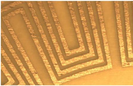
Fig. 4: Detail of a 200µm linewidth and 4 turns copper planar coil on polyimide substrate.
