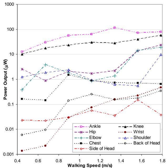
Fig. 7: Power output for a 4-layer coil generator placed on several body locations while walking at different speeds on a treadmill.
