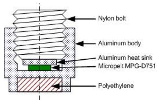
Fig. 2. Cross-section of test article.
