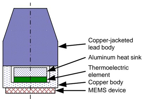
Fig. 5. Cross-section of simulated energy-harvesting projectile.
