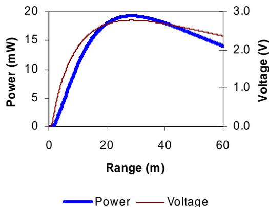
Fig. 6. Simulated power and voltage as a function of distance traveled.
