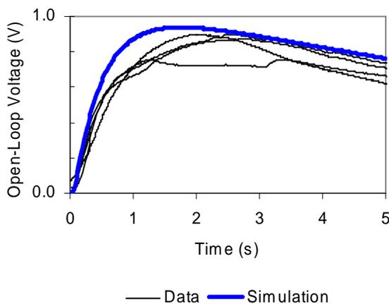
Fig. 3. Open-loop voltage in the test article and in simulation.
