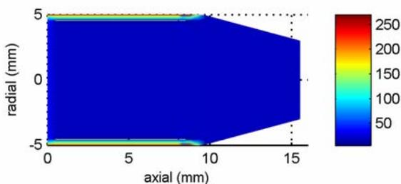
Fig. 1. Temperature distribution in a small-caliber projectile at muzzle exit.
