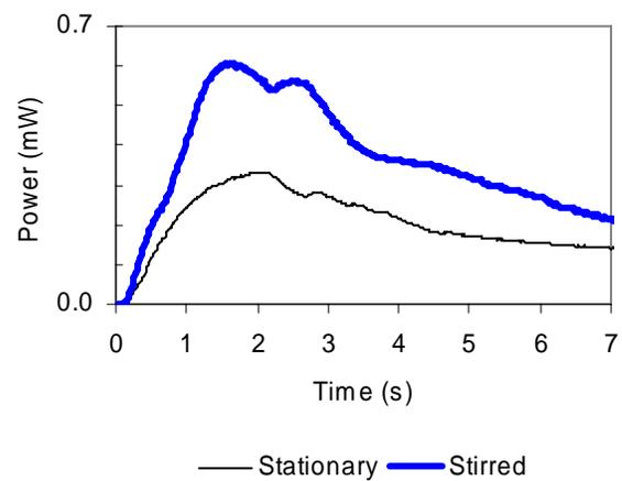
Fig. 4. Power profiles with 509  $\Omega$  load, test article held stationary and stirred in water.
