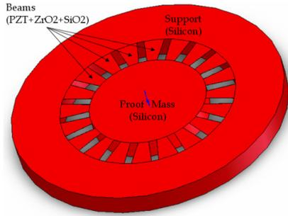
Fig. 2: Schematic structure of wide-bandwidth MEMS-scale piezoelectric energy harvesters.
