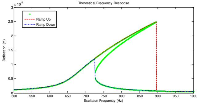
Fig. 4: Theoretical frequency response
