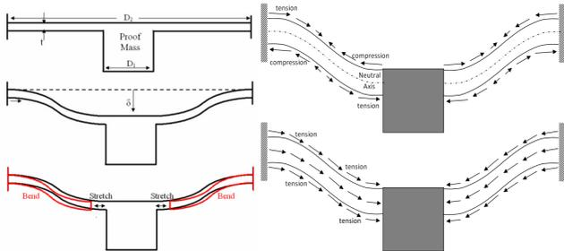
Fig. 3: Bending vs stretching
