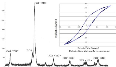
Fig. 7: XRD crystallography and P-V curve
