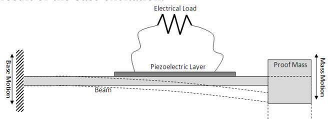
Fig. 1: Traditional design based on cantilever beams
