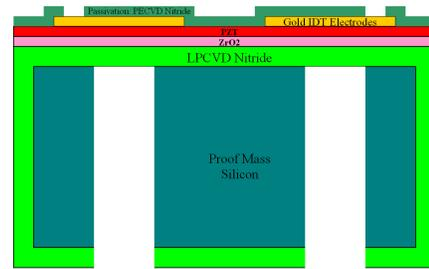
Fig. 5: Schematic cross-section of the device
