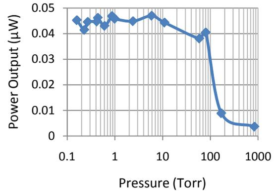
Fig. 11: Effect of pressure on output power.
