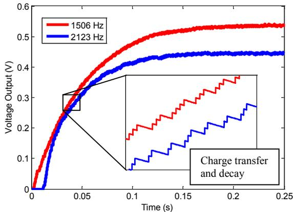
Fig. 4: Simulated output voltage at load resistor.
