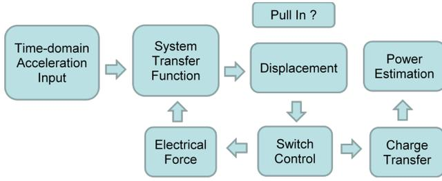
Fig. 3: Flow of the numerical system-level model.
