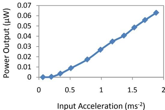
Fig. 9: Plot of output power versus input acceleration.
