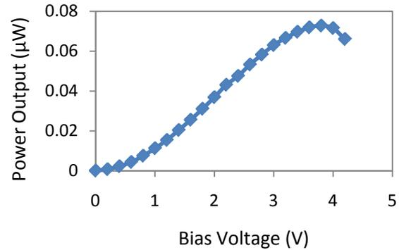
Fig. 10: Effect of DC bias voltage on output power.
