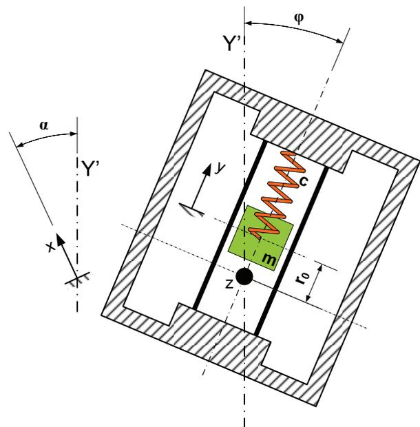
Fig. 1: Concept of the self-alignment mechanism.
