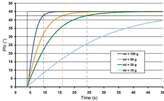
Fig. 6: Step response of the angle  $\varphi$  for different masses; the angle  $\alpha$  was stepped at time = 4 s from  $0^\circ$  to  $45^\circ$ ; in this study the masses  $m_p$  and  $m_c$  were varied at the same time in accordance to a specific scaling factor; the displacement amplitude was kept at 2 mm.
