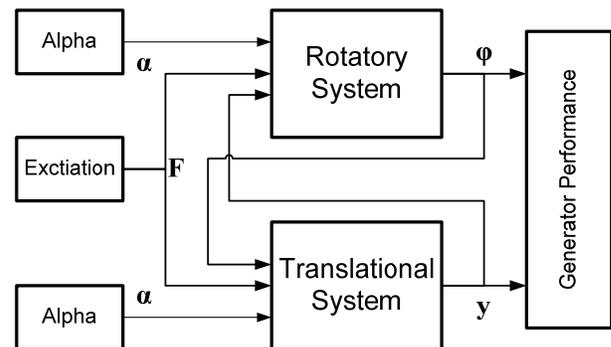
Fig. 2: Schematic diagram of the signal-flow model.
