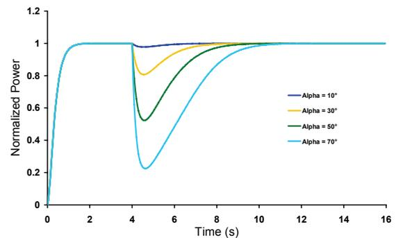
Fig. 5: Step response of the output power of the generator; the angle  $\alpha$  was stepped in the same manner as shown in Fig. 4.
