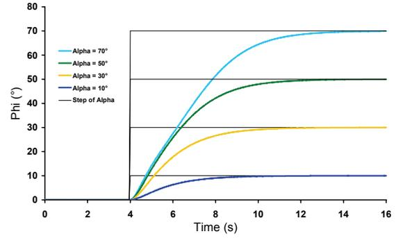
Fig. 4: Step response of the angle  $\varphi$ ; the angle  $\alpha$  was stepped at time = 4 s from  $0^\circ$  to a specific value; the initial value of  $\varphi$  at time = 0 s is  $0^\circ$
