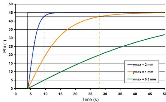
Fig. 7: Step response of the angle  $\varphi$  for different displacement amplitudes; the angle  $\alpha$  was stepped at time = 4 s from  $0^\circ$  to  $45^\circ$ ; the masses  $m_p$  and  $m_c$  were kept at 100 gram.
