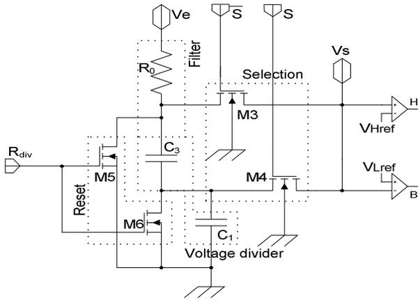
Fig. 5: Capacitive voltage divider implementation.
