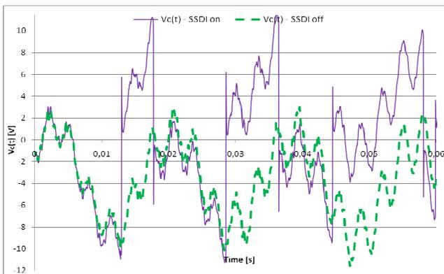
Fig. 8: Piezoelectric voltage  $V_c(t)$  with and without SSDI control.
