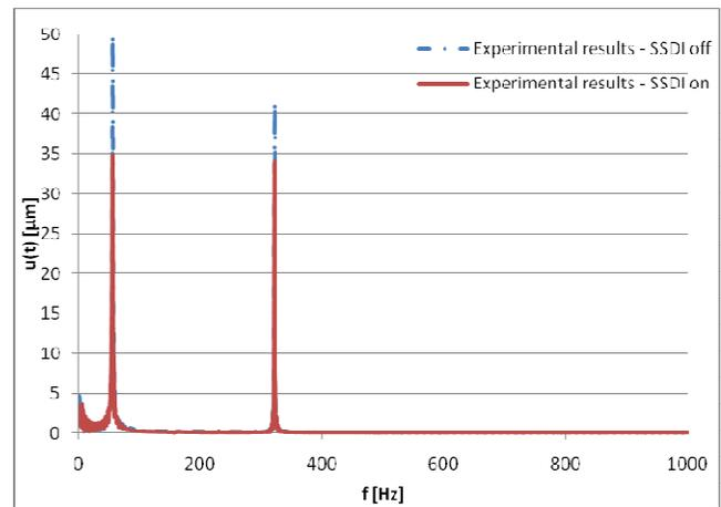
Fig. 9: Measured spectra of mechanical vibration for SSDI ASIC on and off state.
