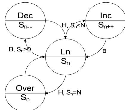
Fig. 4: Finite state machine of the voltage divider.
