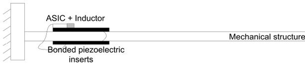
Fig. 7: Schematic of the electromechanical device.
