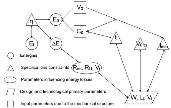
Fig. 2: Effects of main parameters.
