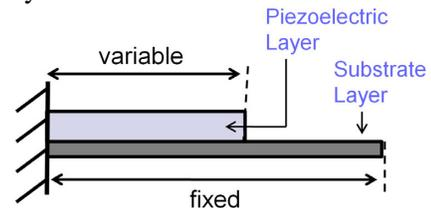
Fig. 2: Adjusting the length of the piezoelectric layer.
