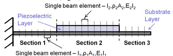
Fig. 1: Non-uniform beam created by moving the piezoelectric layer.
