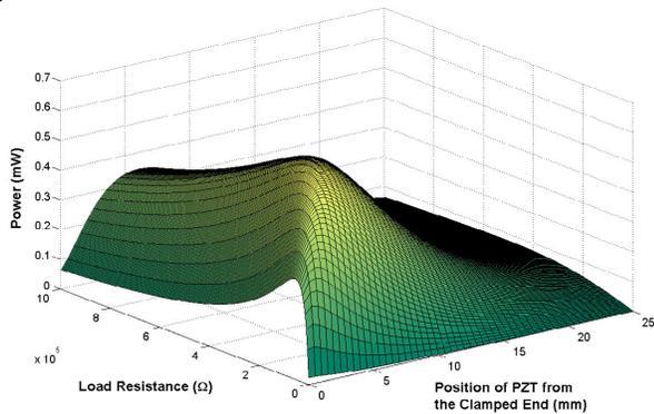
Fig. 4: Trend in power output while modifying the piezoelectric position and the load resistance.
