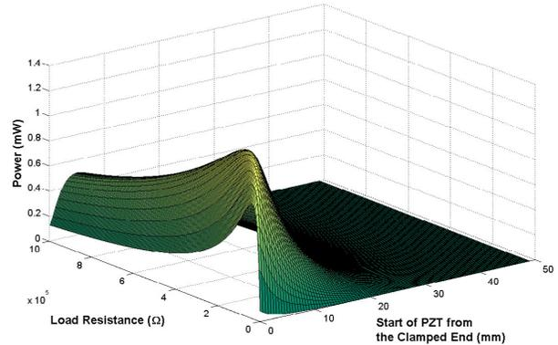
Fig. 5: Trend in power output while altering the piezoelectric start position, thereby changing its length, and the load resistance.
