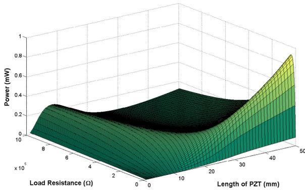
Fig. 3: Trend in power output while modifying the piezoelectric length and the load resistance.
