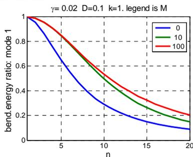
Fig. 7: Effect of tip mass on *BTR*
