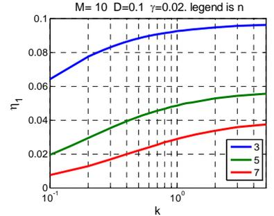
Fig. 4: The effect of  $k$  on the first natural frequency.
