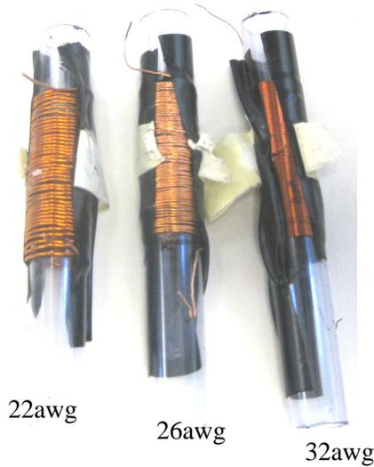
Fig. 2: Three prototype harvesters of varying wire gauge used to test theory.
