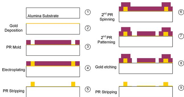
Fig. 5: Fabrication process flow for the bonded chip
