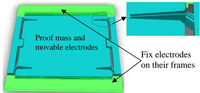
Fig. 1: The 3D layout of electrostatic energy harvester includes two fix electrodes and proof mass suspended by 4 nonlinear springs.
