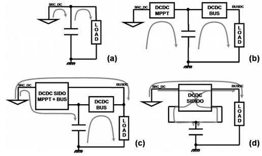
Fig. 3: Architecture of different power harvesting and management systems.
