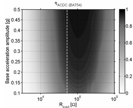
Fig. 4: AC/DC efficiency versus load and vib. level.
