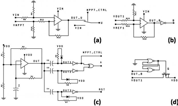
Fig. 6: Schematics of the DC/DC control circuitry.
