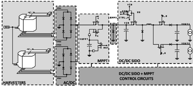
Fig. 5: Schematic of the power chain of the system.
