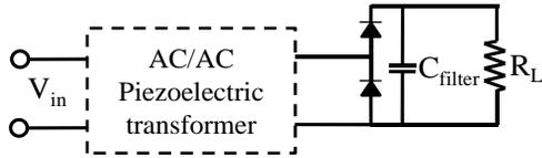
Figure 6: AC/DC PT used in a voltage doubler configuration.
