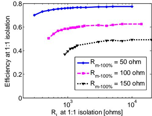
Figure 5: Expected efficiency versus  $R_L$  for 1:1 isolation where each point represents the optimized electrode design.
