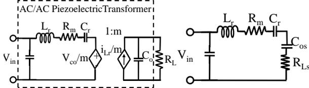
Figure 2: (Left) Small signal series resonant model of the piezoelectric transformer and the load resistance of the subsequent stage. (Right) Illustration of the equivalent parallel to series load.
