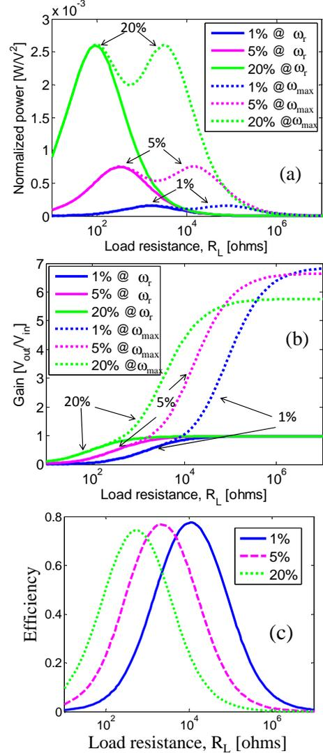
Figure 4: (a) Normalized power delivered to the load, (b) voltage gain and (c) efficiency versus  $R_L$ .
