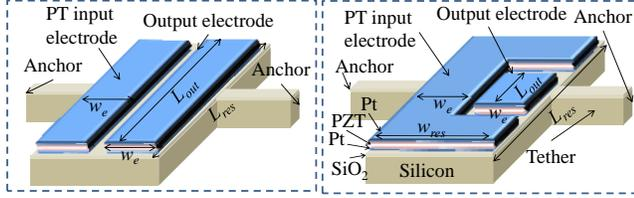
Figure 1: (Left) Illustration of matched input and output electrode coverage in prior art. (Right) Illustration of optimizing the electrode coverage for load impedance matching where the  $L_{out} \times w_e$  area is traded for a larger input electrode area.
