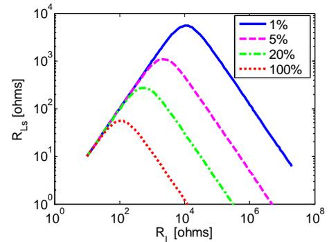
Figure 3: Equivalent series resistance,  $R_{Ls}$ , versus  $R_L$  with varying electrode coverage,  $L_{out}/L_{res} \times 100\%$ .
