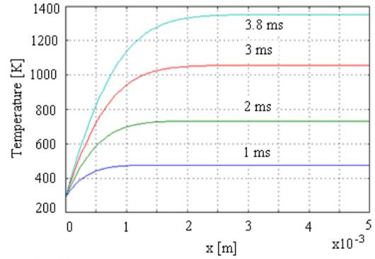
Figure 2. Temperature development through the 10 mm long Cu microwire with 100 um diameter. 5 mm is the center position of the wire.
