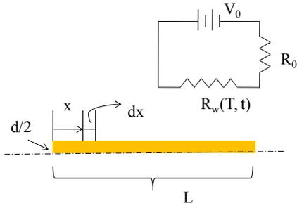
Figure 1. Schematic illustration of the electrical thermal coupled model.  $V_0$  is a voltage source,  $R_w$  is a wire resistance, and  $R_0$  is a sum of all other resistance in the circuit.
