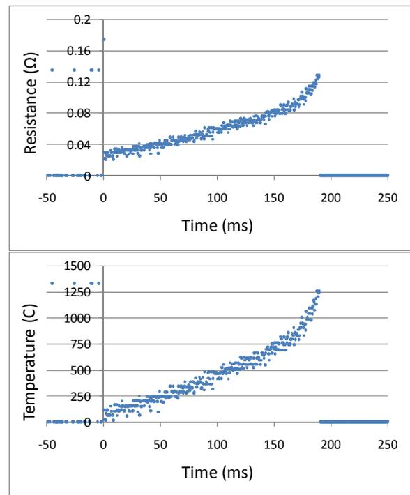
Figure 4. Resistance increases during heating until the wire burns and breaks (top). Temperature increase calculated based on temperature dependence of resistivity (bottom).
