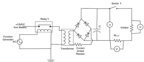
Figure 5. Schematic of the electrical circuit
