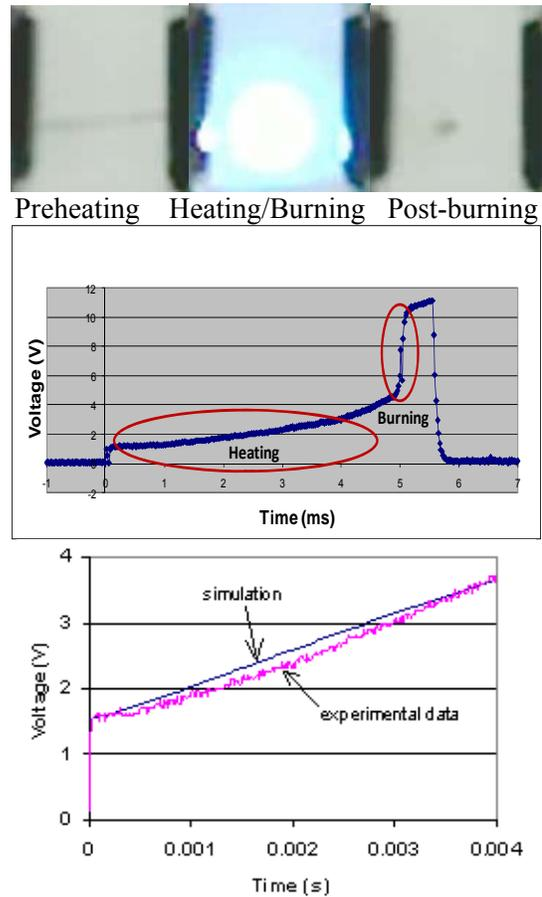
Figure 3. The captured moment of ignition of microwire-based initiator (top). Voltage development of microwire shows heating and burning process by few milliseconds of current flow (middle). The experimental result is in good agreement with a simulated result during heating (bottom).
