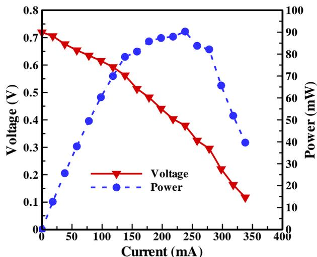
Fig. 7: The Polarization and power curve of the fuel cell without silver deposited on the reactive area
