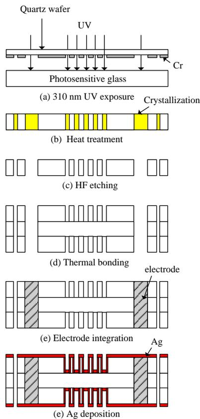
Fig. 3: Microfabrication process of the bipolar plate using glass wafer.
