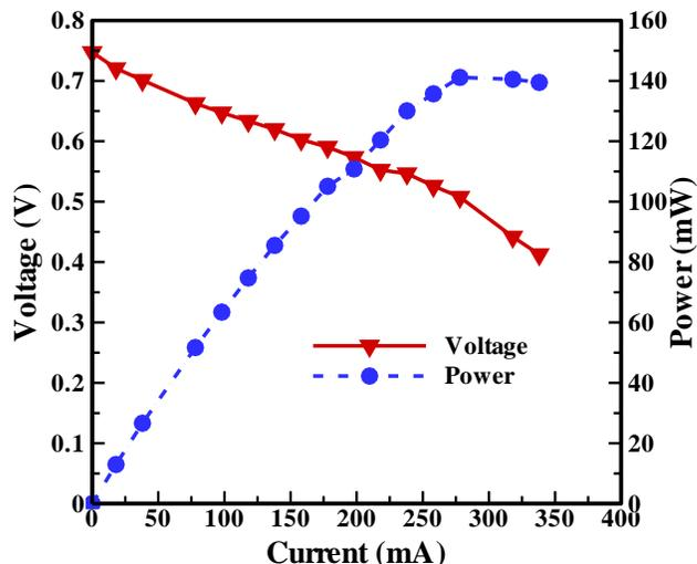
Fig. 6: The Polarization and power curve of the fuel cell with silver deposited on the reactive area
