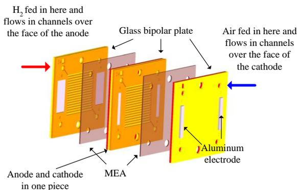
Fig. 1: Schematic of the micro PEM fuel cell stack.
