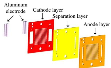
Fig. 2: Detailed components of the bipolar plate.
