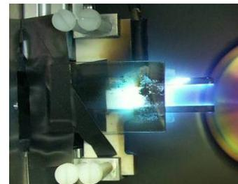
Fig. 3: Prototype  $\mu\text{PPT}$  Thruster During Testing.
