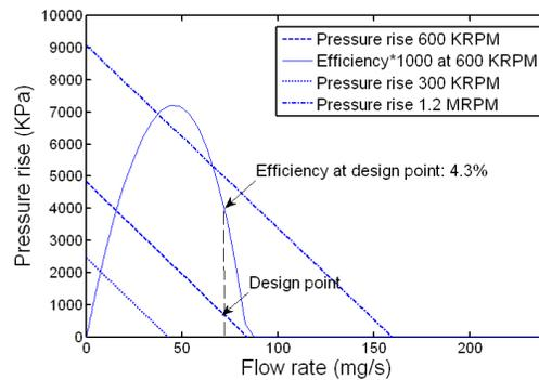
Figure 4: Pump map of pressure rise versus mass flow rate for three different speeds.
