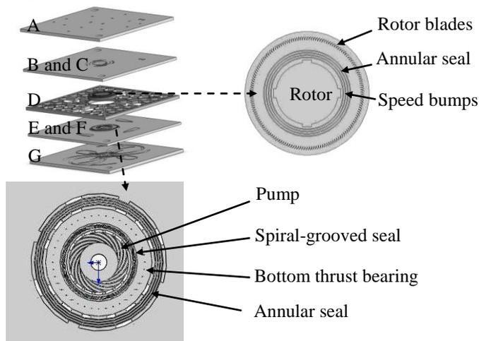
Figure 2: Layers of the microturbopump demo device, in the final version, B is in SOI, D in Pyrex, F in Pyrex. A, C, E and G are in Silicon.
