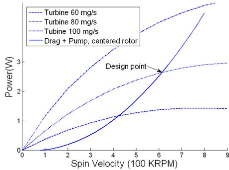
Figure 3: Map of the power delivered by the turbine for several flow rates and comparison with power consumption in the pump and viscous losses.
