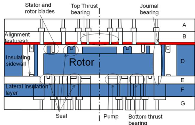
Figure 1: Schematic cross-section of a Rankine Micro turbine. The structure is ~2 mm in thickness and ~15 mm on its side, with a 4 mm diameter rotor.
