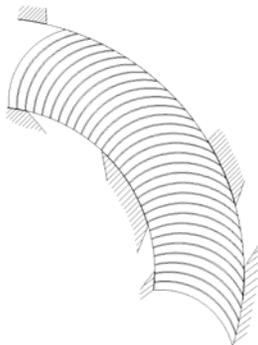
Fig. 3: Schematic of the curved channels and angled porting
