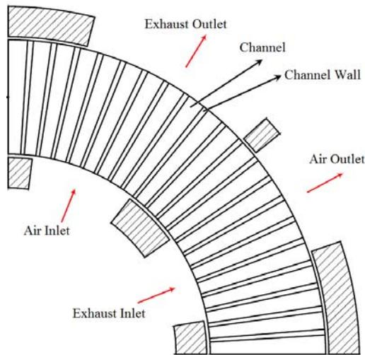
Fig. 2. Schematic of the straight channels and porting
