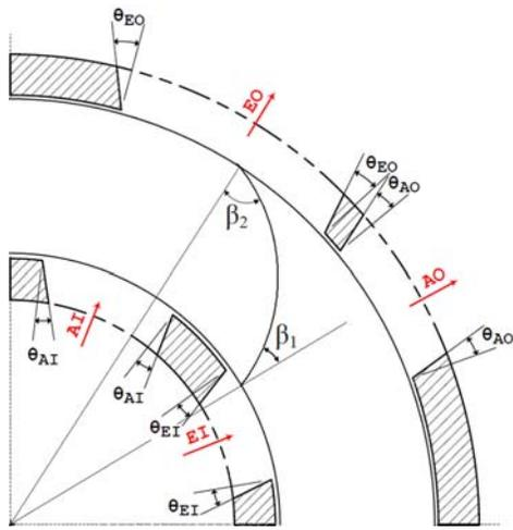
Fig. 4: Schematic of the parameters of the channel curvature and the porting angles for optimization
