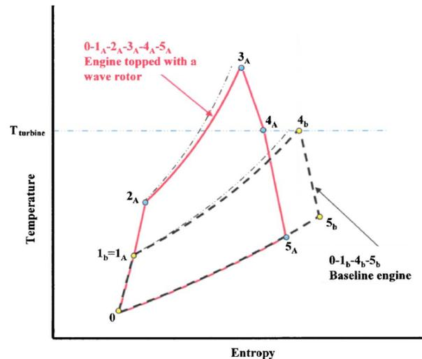
Fig. 1: Schematic  $T$ - $s$  diagrams for a gas turbine baseline engine and the wave-rotor-topped gas turbine
