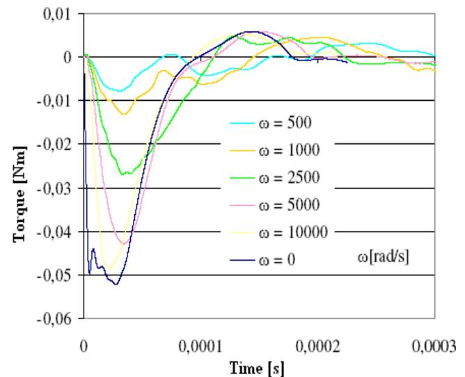
Fig. 4: Relation between the disk speed and torque developed during the expansion process
