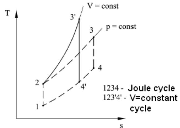
Fig. 1: Comparison of the Joule cycle with the constant volume combustion cycle in a T-s diagram
