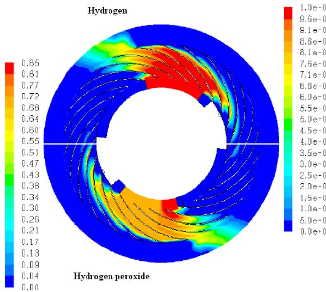
Fig. 8: Contours of Hydrogen and Hydrogen Peroxide Fractions
