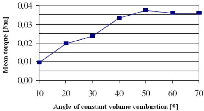
Fig. 9: Relation between the Torque Generated and the Angle of Constant Volume Combustion
