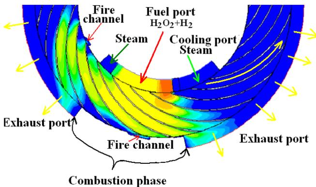
Fig. 2: Cycle Schematic of lower half of a two cycle per revolution Radial Disk Internal Combustion Engine.
