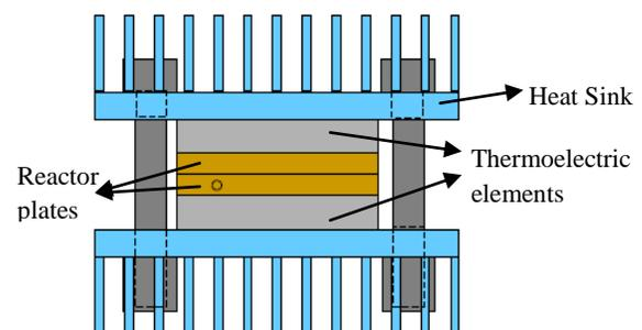
Figure 1: Schematic of integrated thermoelectric/ microcombustor device shown without any thermal insulation.
