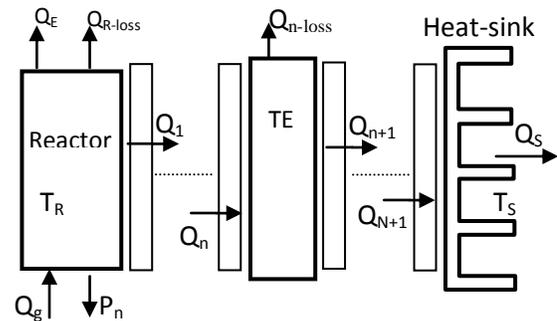
Figure 3: Schematic showing the flow of energy on one side of the integrated device.
