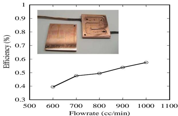
Figure 2: Efficiency of the integrated device vs. the total gas flow rate through the microcombustor. Inset shows a photograph of the serpentine channel microcombustor used.
