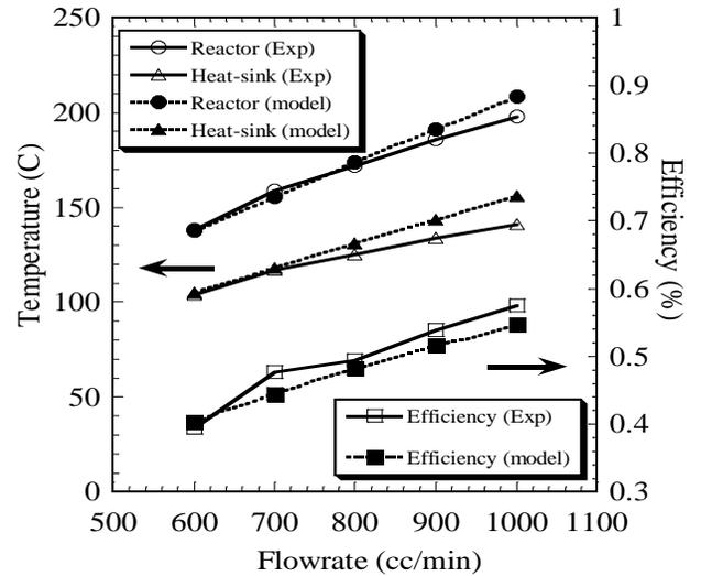
Figure 4: Comparison of the experimental and model values of reactor temperature, heatsink temperature and device efficiency.
