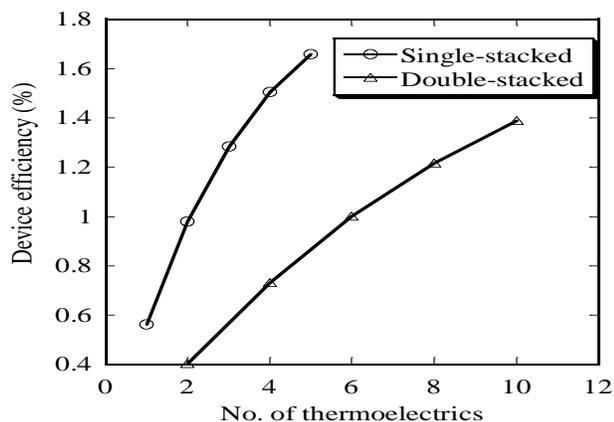
Figure 5: Device efficiency of single-sided stacked and double-sided stacked arrangements as a function of the total number of thermoelectric devices.
