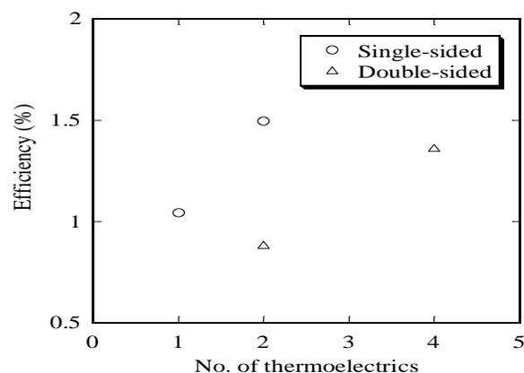
Figure 6: Experimental device (with ceramic heater) efficiency of single-sided stacked and double-sided stacked arrangements as a function of the total number of thermoelectric devices.
