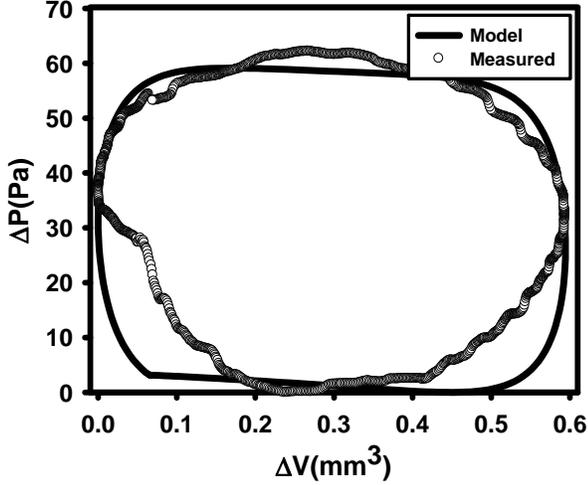
Fig. 2. P-V diagram of resonant operation.
