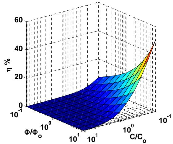
Fig. 3. First-law efficiency versus thermal inertia and time-geometry factor.
