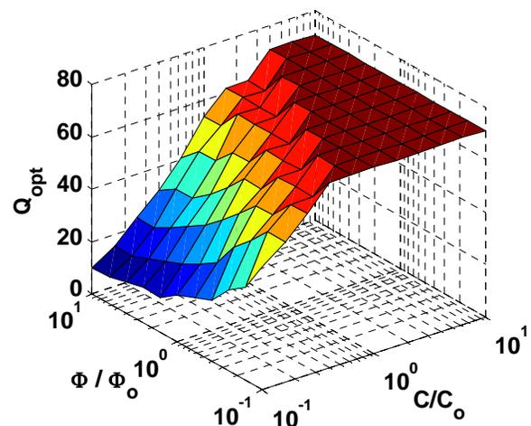
Fig. 4. Optimal quality factor versus thermal inertia and time-geometry factor.
